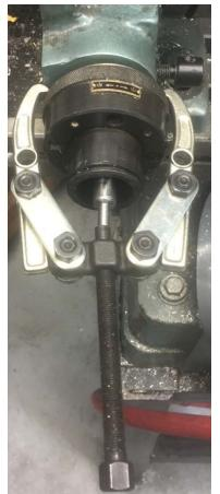
This was the once place where the *dis*assembly was a bit tricky. I figured out that I needed to use a gear puller on the collar after removing the screws.
