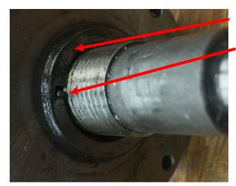
The washer with a slot cut into its inside diameter slid neatly over the bent wire so it locked to the shaft and could not rotate.
