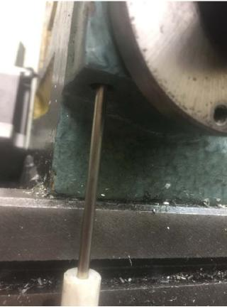
The rounded end set screw threaded into the bottom hole first. It took a lot of turning before it contacts the axial stop.
