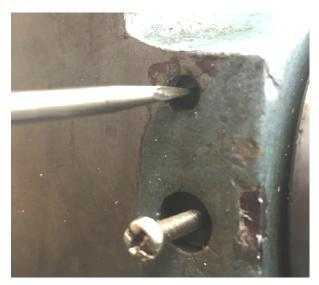
I knew I had installed the correct set screw because, when tight, the face was just below the surface of the casting.
