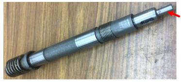
Here is the driveshaft after I turned down the threaded end. Because the part was originally turned between centers, it was easy to put it back on centers and accurately turn down the end on my lathe.
