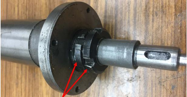
Then I screwed on the two nuts finger tight. Final alignment and locking took place later.
