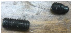
I found these two set screws. The longer set screw was used to lock on the graduated collar but I will use it to better lock the smaller set screw.
