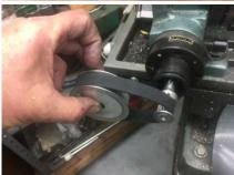
With the rotary table reassembled, I was able to attach my small sprocket and start to design how the belt and large sprocket will be attached.
