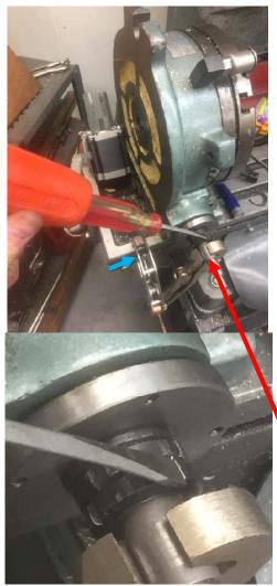
This next step was to remove most of the axial movement of the shaft. I first tighten the two nuts together so they locked using a pair of Channel Locks. The trick was to have a gap between the disk and the inner nut. Then there was room to grab this nut.
