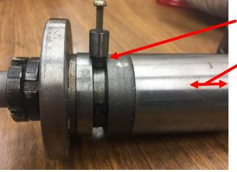
The flat part engages with the groove and is tapered so when snug, the shaft carrier does not slide in and out.
