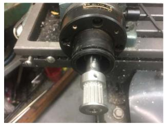
My goal was to install a cog belt sprocket on the end of my horizontal/vertical rotary table's drive shaft. This required me to remove the shaft, turn the end down on my lathe, and re-install.
