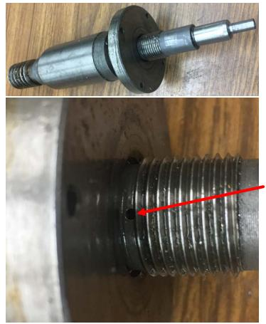
The shaft slid into its carrier. It is a close sliding fit. If the shaft doesn't slide in easily, take it apart and check for swarf.
