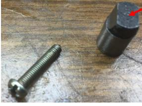
I located this part and called it an **axial stop**. At least in my case, there was a hole in the other end that was tapped. I found an odd screw that fit the hole.
