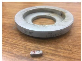
There were two pieces left over. The calibrated ring is a press fit over the collar. After removing the set screw, I used the gear puller to slide it off.
