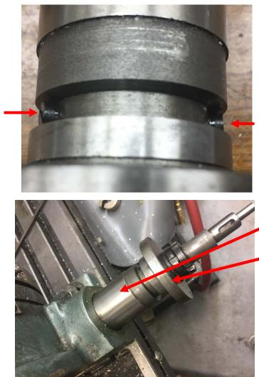
Here the two radial stops are installed and tightened down.
