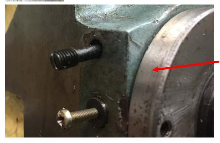
I slid the gear stop into the hole just above the radial stop.
