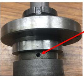
I located two holes in the groove behind the disk. Here is one of them. The other is about 120° off from it.
