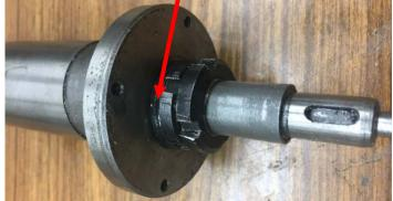
Once the nuts were locked together, I clamped the shaft in a non-critical area. In my case, it was in front of the nuts because the turned down section must be preserved. Note the Kant Twist clamp that acts as a stop for the Channel Locks (blue arrow).
