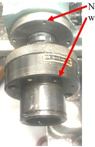
Next, I aligned the holes in the disk with the holes in the collar.
