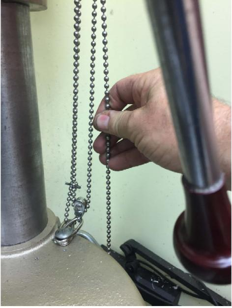
When I want to adjust the table, I unlock the column clamp. Then I pull on the ball chain going to the counter weight. A slight pull down and the table rises. A slight pull up and the table lowers. When done, I check the tables rotational position and then relock the table.
