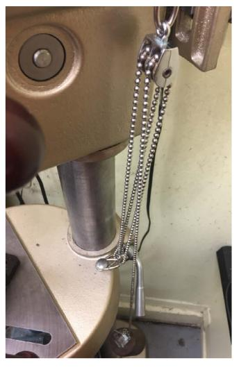
Using miniature pulleys plus some ball chain, I rigged up a little block and tackle. At the bottom of the picture you can see the top of my counterweight. The ball chain pulls up on the table near the column with about as much force as the table pulls down when it has my vise on it and is unlocked.
