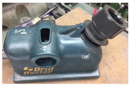
I have owned this Drill Doctor for 16 years and am very happy with it. About 5 years ago I replaced the diamond grinding wheel. Now the collet has become hard to turn. Before I buy a new collet for \$35, is there a way to fix what I have? Nothing to lose.
