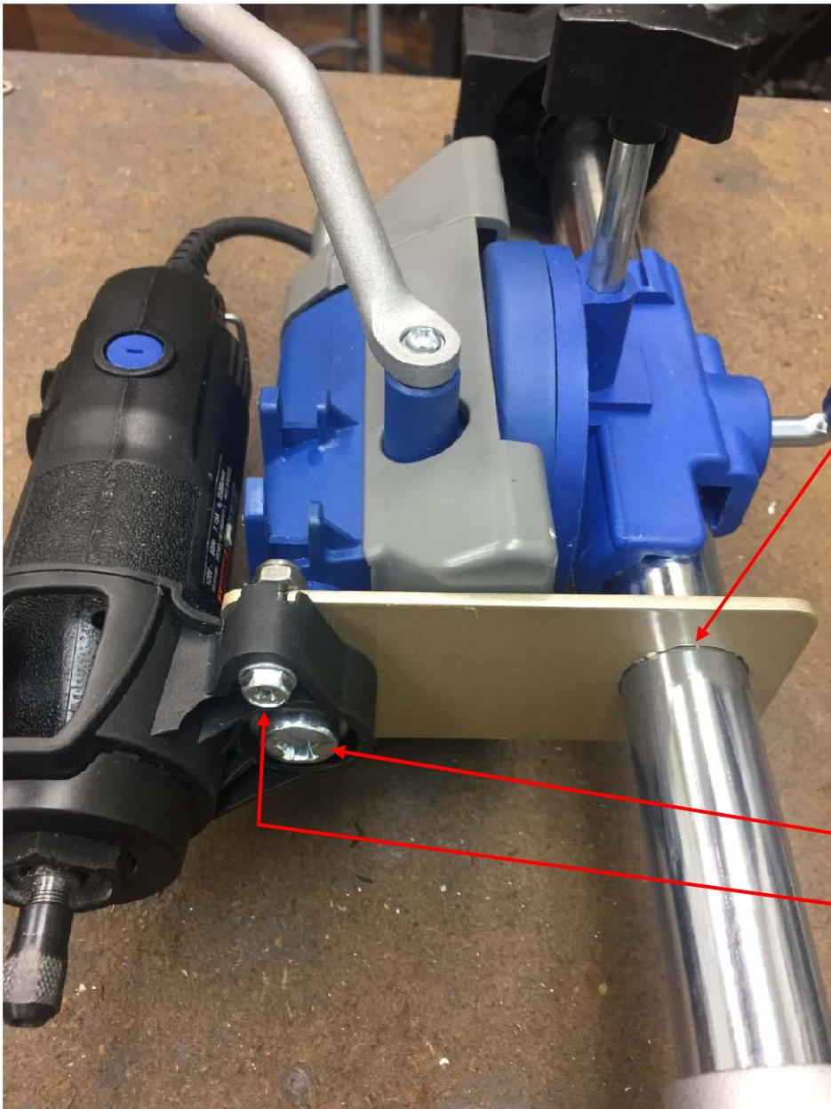
My solution was to increase the distance from the center of ram to the point that stops the rotation. This was done by fabricating a plate from  $1/8" \times 1 \frac{1}{2} "$  aluminum plate. One end was step drilled<sup>2</sup> out to 1". It is a sliding fit on the pillar.
