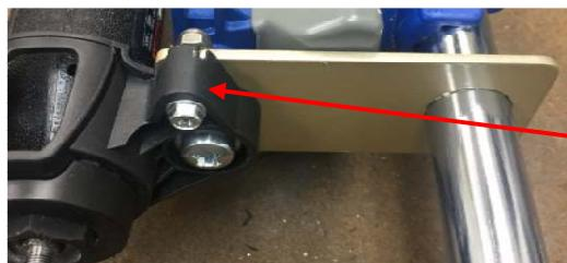
With the plate on the pillar and the large screw securely in place, use the plastic flange to guide a drill into the plate. Select a drill bit that is a close fit to the plastic hole. You only need to drill in enough to cut a cone. Then remove the plate and finish drilling the hole. This is much easier than trying to exactly locate this third hole.
