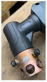
My solution was to fabricate a cylinder that replaced the wire standoff. It slides over the ceramic cone, and three screws lightly engage the existing groove.
