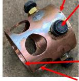
Using a 29/64-inch drill<sup>3</sup>, I drilled a series of holes at the other end of the cylinder. My goal was to have about 0.1 inches from the bottom end of the cylinder to the bottom of each hole.
