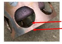
Then I trimmed the overall length of the pipe so the tip of the cutter was back from the bottom edge by the same distance as seen with the wire guide, while the top of the pipe was flush with the top of the ceramic.
