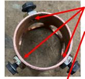
I drilled three #36 holes about 120° apart and tapped them 6-32, using the ceramic sleeve as my guide for the distance from the top edge of the cylinder to the center of the groove.
