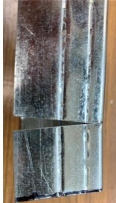
Then I use a tin snips to cut a V on each side at the first mark. The V provides a bit of room as the end section is bent up.
