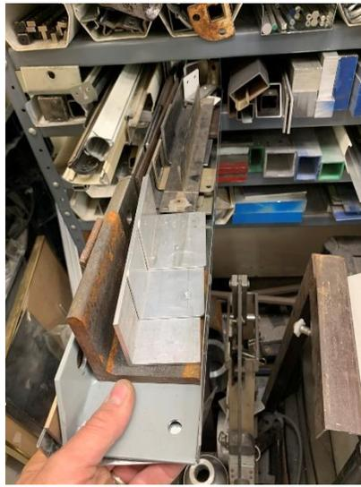
See my nice pull-out custom drawer? It is 3 ½ inches wide and can be any length up to 10 feet. The cost is about \$1.00 per foot. The icing on the cake is that you only need a tin snips and a pliers to make it.
