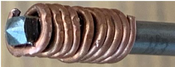
The next time you need this tool, slide the copper sleeve back onto the tap.
