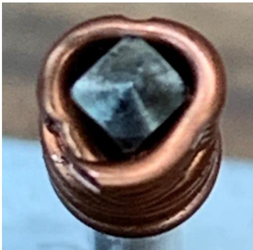
Can we relax the requirement a bit? Using some copper wire, I was able to form it close enough to transmit rotational force and be reasonably well centered.
