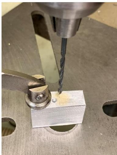
Next, I positioned my part and put the tap drill in my drill press chuck.
