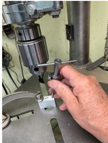
You may quickly run into problems. The tap, mounted in its handle, can't fit between the chuck and the part.
