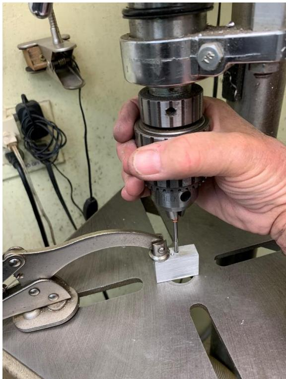
After introducing some tapping fluid into the hole, I fed the quill down with one hand until it contacted the part. I then used the other hand to turn the chuck one revolution. The tap was then bedded enough to counteract the upward force of the quill retraction spring. It was then easy to turn the chuck and cut the threads with one hand.
