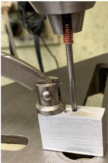
Place the point of the tap in the hole, lower the jaws, and lock the vertical position. Slowly rotate the tap's shank with one hand while gently closing the jaws with the other hand. The jaws will find the flat spots. Then fully tighten the chuck.
