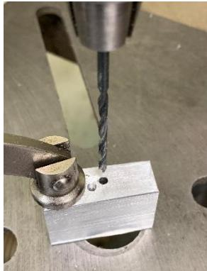
The best time to run a tap is right after the tap hole has been drilled. All is in alignment, and the chuck can drive the tap. Well, almost true.
