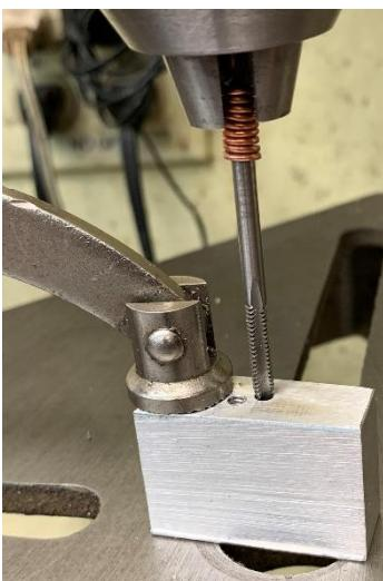
After drilling, I removed the drill and opened the jaws to accept the modified tap.
