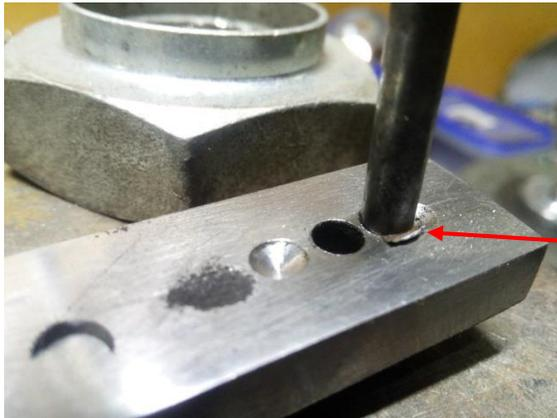
A piece or close fitting rod was forced through the guide pin hole.
