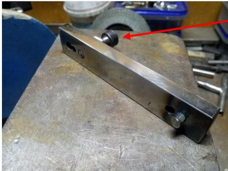
After deburring, a bolt with a nut threaded on was screwed into the hole. The nut was then tightened. Finally, the bottom of the screw was ground flush with the bottom of the bar. I didn't want anything catching as the bar was rotated during use.
