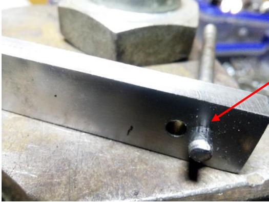
The pin extends out the bottom enough to securely engage the hole to be drilled in the part.
