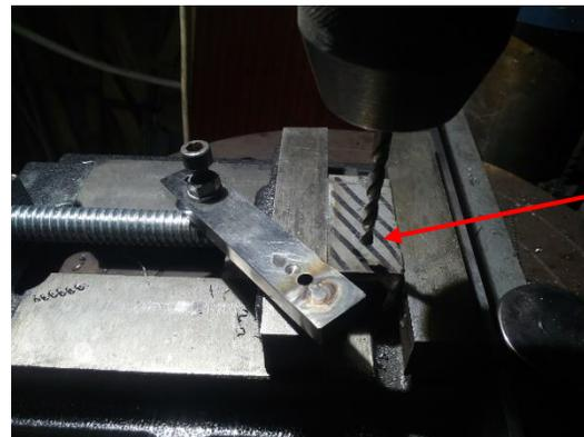
To use the tool, first drill a 4.2 mm hole in the part.
