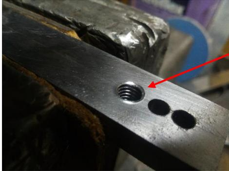
The hole was tapped M6. Given how tough the metal is, lots of cutting oil was used and I went slow. It would have been easy to snap even this large tap off.
