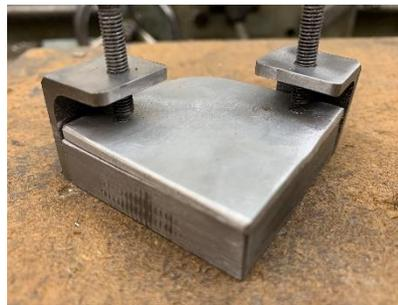
This tool permits me to file a 7/8<sup>th</sup> inch radius on a plate that is at least 2 inches by 2 inches. No holes are drilled in the stock. Instead, those two build-in clamps secure the tool to the stock.
