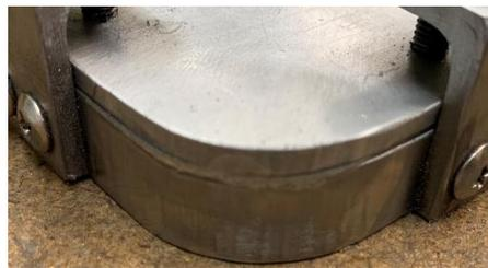
Here you see that the excess stock has been abraded down to the curved surface of the base.
