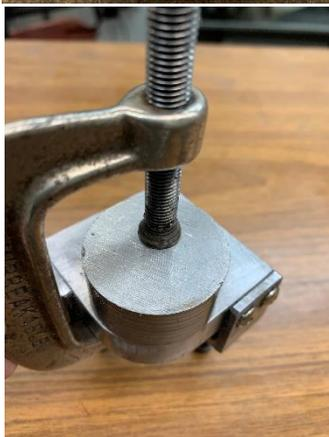
Karl\_H of [homemadetools.net](http://homemadetools.net) had an excellent question: how did I made the radius on the base? I took a piece of round stock 1 1/4" in diameter and clamped it to the base. Then I used a grinder followed by my belt sander to form the rounded corner on the base. So to make a button, you need a button. Thanks Karl.
