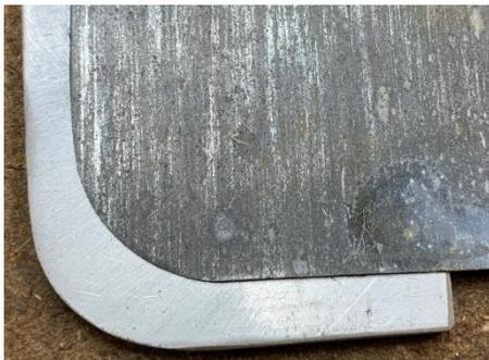
After deburring, the corner of the stock is a good approximation of a 7/8<sup>th</sup> inch radius.
