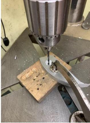
Next, I chuck up a 1/8<sup>th</sup> inch drill. Using the bottom of the cone for alignment<sup>2</sup>, I drill through. The custom tool is done.
