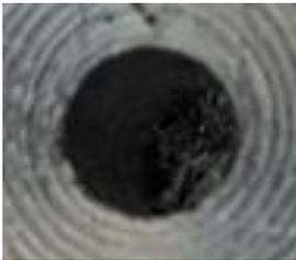
I had previously faced this piece in my lathe, and you can see a series of concentric circles that confirm the hole is centered fairly well. The hole should be as well centered as the point of the 1/2-inch drill.
