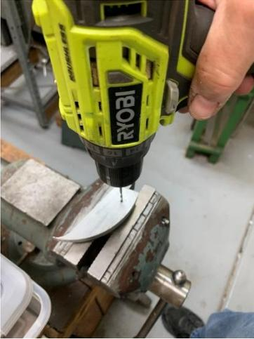
With my 1/8<sup>th</sup> inch drill chucked into my hand drill, I use my custom tool as a form of bench block. It gives axial and radial alignment.
