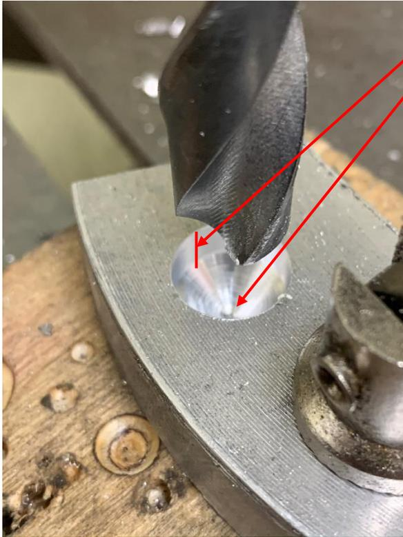
I want to have at least 3/16-inch of bore. The drill will provide a cone at the bottom of the hole.
