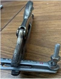
After starting the nut by hand, I drive it down and back up with my electric screwdriver. The bolt is pulled out of the tool and tossed into a bucket.
