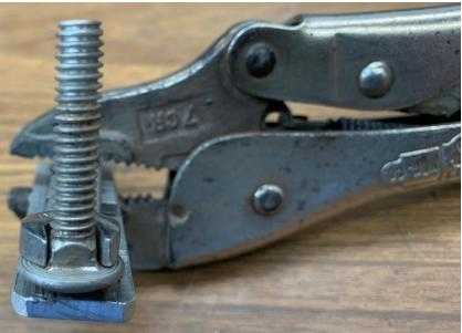
The stack consists of the wrench, a spacer, and a piece of aluminum. By clamping at a distance from the end, I can use the flex of the aluminum to clamp the head against the wrench. It is strong enough to hold yet easy to release.
