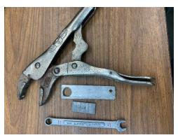
I used a metric wrench that fit the tapered square shank of the carriage bolt good enough to stop rotation. Added two pieces of scrap metal and a vise grip, and I was ready to go.
