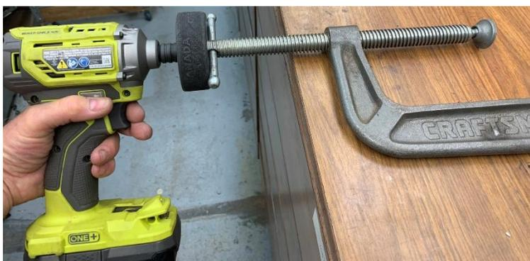
With the crossbar approximately centered, I push my "Speed Drive" against the end of the threaded rod. By slowly pulling the trigger, the clamp quickly adjusts to the desired position.
