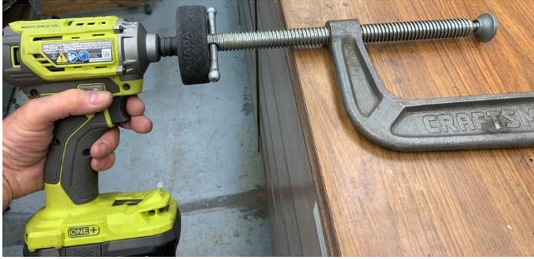
With the crossbar centered, push the tool against the top of the threaded rod. The bored out hole provides clearance for the top of the threaded rod. The soft surface of the puck contacts the crossbar to prevent side motion while also enabling the turning puck to couple with the threaded rod.
