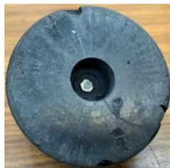
the other end of the hex drive is flush with the bottom of the bored out hole in the puck.
