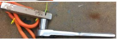
Then the wrench turns the bolt and winds up the tail of the tie. You must judge how tight to make it. Too tight can damage the cable.
