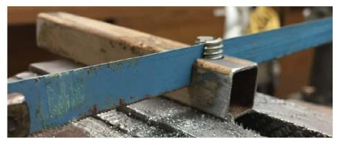
Cross drilling the steel ½" x ½" tubing with a 3/8" drill. Then fit the tubing over the bolt which is still clamped in the vise. Use the hacked hacksaw to cut down to the bottom of the existing slot.
