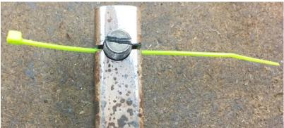
With the bolt in the tubing and the slots aligned, a cable tie can be slid inside.
