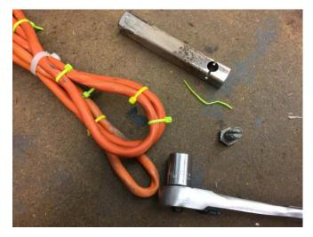
When the tie is tight enough, unwind the tail from the tool and cut it off.
