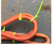
The first step is to attach the cable tie and pull it snug by hand.
