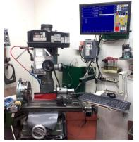
What excited me about having Screw Mapping as a Centroid CNC12 feature was the hope of improving the accuracy of my lead screw driven RF30 Mill/Drill.
