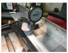
Now consider what happens in this example when we use a distance *setting* device like a stack of gage blocks<sup>16</sup> and a DTI.
