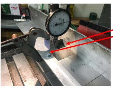
Slide the stack of blocks into the finger of the DTI until it reads  $0 \pm \frac{1}{2}$ . Tighten the clamp.
