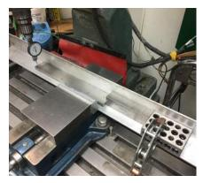
First Home the machine. Then put a finger DTI in the chuck. I used a Mitutoyo DTI that reads from -15 to +15 thou with a resolution of better than a tenth. Turn the bezel so the needle points to about -5. Be sure the finger moves back and forth parallel to the X axis and that the spindle does not rotate.
