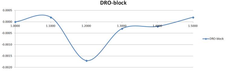
Here is a closer look at compensated X axis movement from 1.000 inches to 1.500 inches. Data has been taken every 0.1000 inches. I fitted a curve just to make it easier to see the data points.
