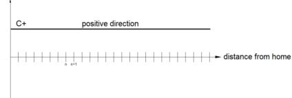
Next consider the effect of constant backlash. As I move in a positive direction, the Screw Mapping data returns a constant value. Call this value  $C_+$ .
