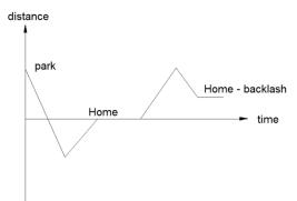
For example, after park, I will be at an X of +0.012 inches. When I home, we move in a negative direction until we are at about -0.012. Then we move in a positive direction to 0.0000. So when initially at Home, the previous direction was positive.
