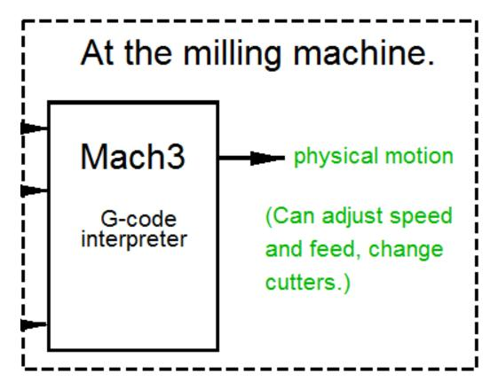
Mach3 accepts text files containing G-code and interprets it to physically operate the CNC mill. Mach3 also accepts limited manual intervention so parameters set in CamBam can be adjusted.
