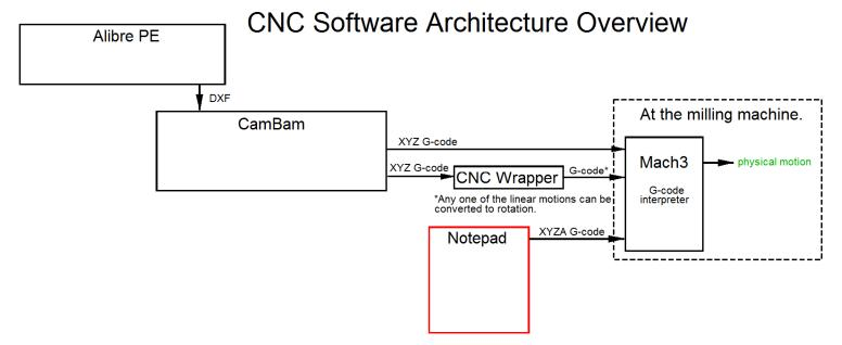
**Alibre PE** lets me generate 3D renderings of parts. It can output one or more *Drawing eXchange Format* (DXF) files that represents 2D views of the 3D part. **CamBam** converts each DXF into a 2 ½D G-code file. **Mach3** interprets the G-code and operates its CNC milling machine. Optionally, **CNC Wrapper** can take the G-code from CamBam and convert it into a form that permits engraving onto cylinders. **Notepad** permits me to hand generate G-code which is acceptable to Mach3.
