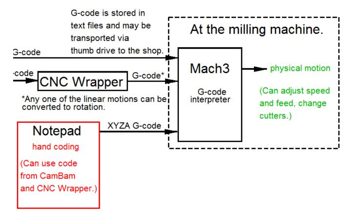
It is common to watch the CNC mill operate and see a need to change something. Sure you could go back to Alibre and make the change. Then re-input all of that data into CamBam to generate new G-code. Maybe you are much more careful than me and do not inject new bugs. Or maybe you are as careful as me and only inject a few new bugs. Either way, it can become one step forward and two steps back.
