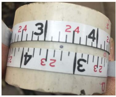
Turning the pipe around, I find the point that is equal distance from the same number. In this case it is about ¼ inch beyond 3 on both tapes. Mark this spot and drill the hole.
