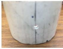
I started by marking a longitudinal line through each hole.
