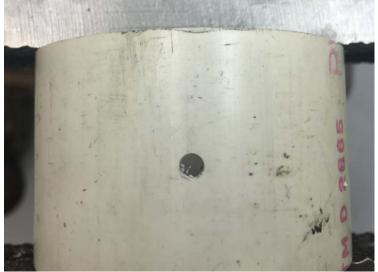
First I drill a hole in the pipe.
