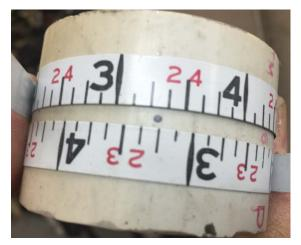
With the two ends of the tool wrapped around the pipe, it will only sit flat if it is square with the surface. This insures radial alignment<sup>2</sup>.
