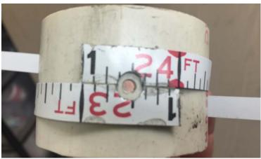
Then I center the hole in the cross drilling tape on the hole I just drilled.
