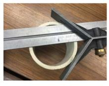
Using a center finding scale, I verified I was on a diameter.
