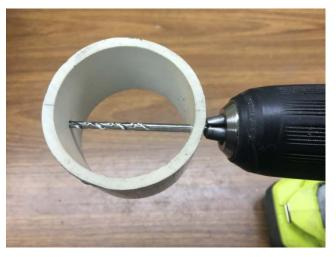
When I need to cross drill a piece of pipe, there are two options. I can pull out my V block, align it under my drill bit set in my drill press, and accurately cut the hole. Alternately, I can eyeball it and be off an unknown amount.
