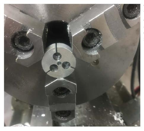
The crush collet has been spot drilled, drilled through with a #32 drill (0.116" diameter), and then reamed to 0.125".
