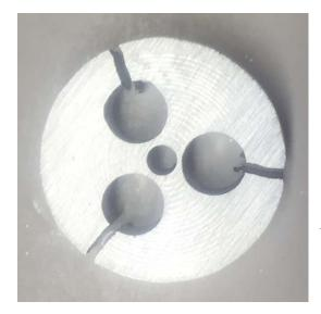
One solution is to make what I will call a "Crush Collet". The solution to re-cutting the center hole is to not have it in the first place. Instead, I drilled 3 holes around the center hole and then made 3 saw cuts. This weakened the collet such that the full force of the 3 jaws can distort the remaining metal and slightly close the center hole. With the jaws snug, I can slide the part into the center hole. When fully tightened, the part is solidly clamped.
