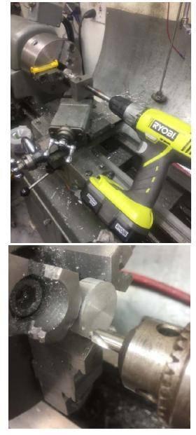
The breakthrough in making the 3 perimeter holes at the same distance from the center was to use my compound mounted drill chuck. I used a line level to set the angle.
