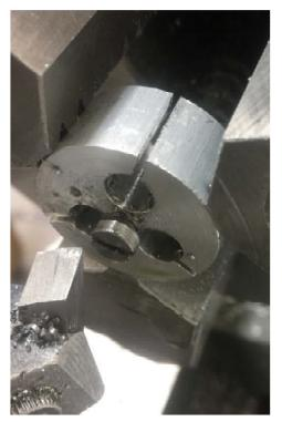
Although my test collets have a smooth hole in them, the real value is when the hole is tapped. It then becomes possible to hold threaded stock like small brass screws without causing damage. Here I have machined the head of an 8-32 screw. It started out with a round head. I saw no unscrewing while machining.
