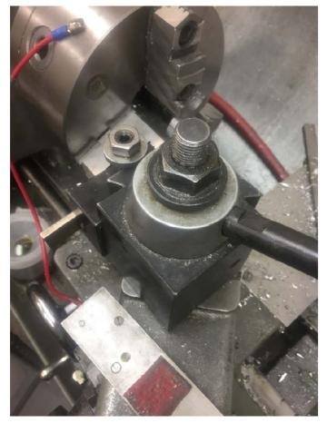
I measured TIR by using my parting tool as a probe. My Electronic Edge Finder<sup>3</sup> told me when the tool contacted the dowel pin. I took readings at 0°, 120°, and 240°. The crossfeed dial told me movement. Then I checked at 60°, 180°, and 300° to verify I had found maximum and minimum.
