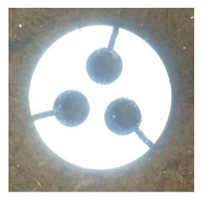
Next I removed the part and drilled through using a <sup>1</sup>/<sub>4</sub>" drill on the drill press. The 3 cuts were made on my bandsaw. It is essential that the saw not slip and cut the far side of any hole. I spoiled one part that way. This caused excessive TIR.
