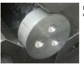
I drilled a starter hole, rotated 120° and drilled the next one. This guaranteed the best possible symmetry.
