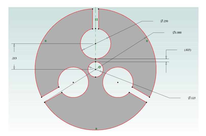
Here is my test crush collet. I used a 1/8" center hole so I could fit it with a 1/8" dowel pin in order to accurately measure TIR. I chose a wall thickness of 0.025" between the nominal position of the center hole and perimeter holes.
