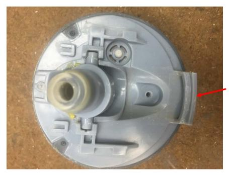
Here is what is under the top cap. There are a number of horizontal tabs that engage with tabs in the top cap. By sliding the top cap away from this large side tab, it will lift off.
