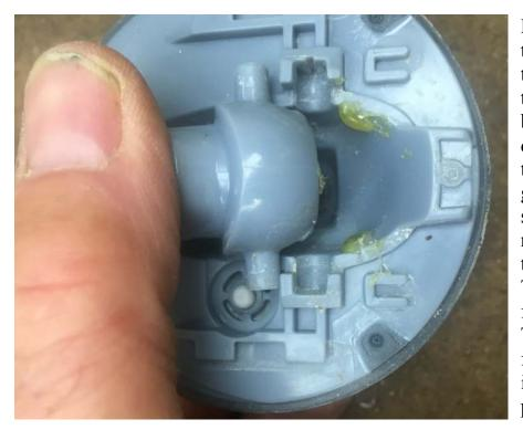
Here is the main trick to the repair. Unsnap the valve to expose the worn out friction bumps. Then put a dab of heat glue on these bumps. Let the glue cool for a few seconds and then reinstall the valve in the lock position. This will properly form the heat glue. Then let the glue fully cool with valve in the unlock position.
