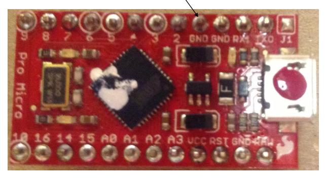
Ground from the caliper connects to GND on the Pro Micro.
