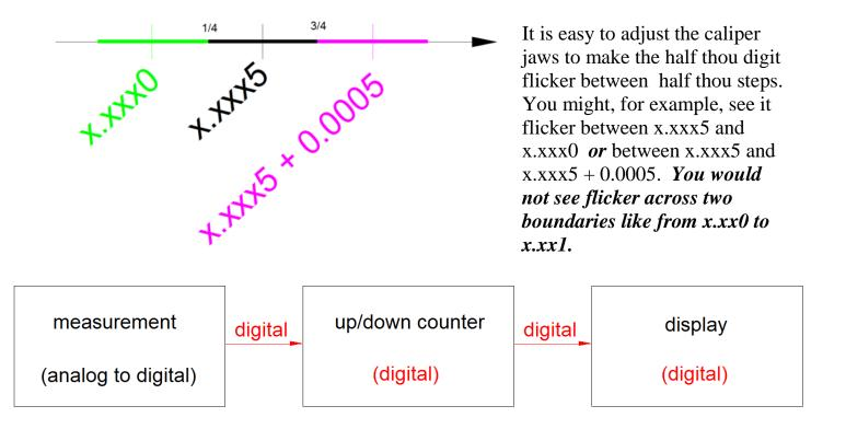
Recall that the measurement function has jitter which will drive the up/down counter to move up and down one step. This flicker means that the up/down counter is sitting right on a transition point of the display.
