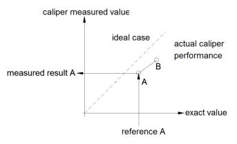
Say I measure a known reference called "A" and note the measured result. Repeat for reference B. This defines a range of values between A and B. If I measured an unknown that really was equal to reference A or B, I could apply exactly the correct compensation to the measured result. Between A and B, I can estimate the correct correction factor. The closer A
