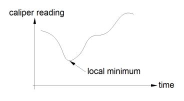
As the jaws close, the caliper reading shrinks in value. Then the jaws contact the workpiece and they can't close anymore. This is the point of local minimum. When the jaws start to open, the caliper reading rises. The program records the caliper reading 8 times per second looking for this local minimum. When it sees it, that value is recorded.
