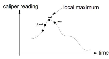
Each time a data point is recorded, the time is also saved. When the software sees a reversal in direction of the data, it knows the middle one is the local minimum or maximum. You see here a data point marked "new". It was just recorded. About 1/8th of a second before it the data point "old" was recorded. About 1/8th of a second before "old", "oldest" was
