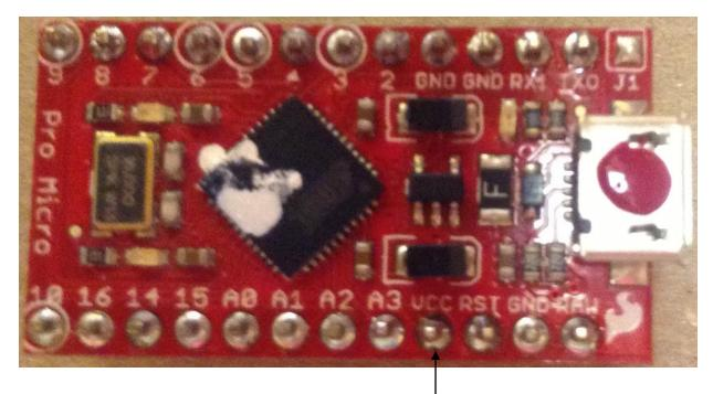
+5V to the caliper interface connects to VCC.
