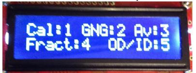
take up to 10 measurements of the same thing and the program will average the result and round to the nearest half thou. This further improves system accuracy. This feature has been designed but not coded yet.
