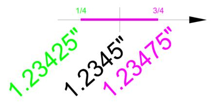
For example, say the caliper displayed 1.2345" and the only error was due to this limitation in the display. Then the actual measured value could be anywhere between 1.23425" and 1.23475". If the actual measured
