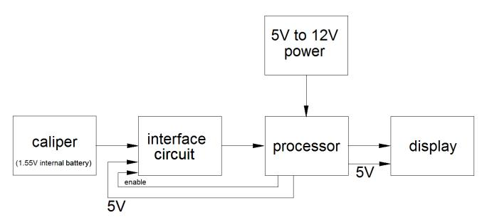
There is also an interface circuit consisting of two general purpose NPN transistors and four resistors. If you chose the Pro Micro 3.3V/8 MHz and 3.3V LCD, this interface circuit probably should not be needed. Minor software changes would be needed to compensate for the clock and data inversion.
