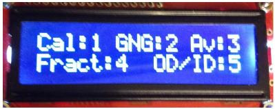
If the user presses the inch/mm button while the UL/CMD is displayed, they are offered a choice of features. Opening the jaws to around 1" selects the calibration mode. This enables the user to measure a series of
