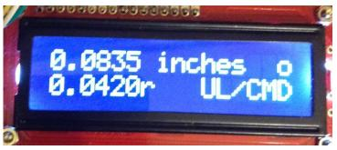
The default display shows decimal inches in the upper left hand corner. Below it is half the value rounded to the nearest half thou. If you use a lathe with in-feed dial in radius, then you can zero the jaws of the caliper at the target diameter and this will
