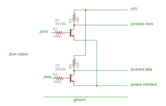
All resistors are 1/8 watt 10%. The two NPN transistor can be any general purpose devices.
