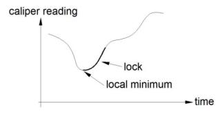
Here you see automatic lock enabled after a local minimum has been detected. Lock is disabled when the caliper readings have increased more than 0.100" from the local minimum reading. It would have also unlocked if the jaws have been closed by more than
