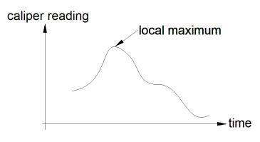
This is the twin of Automatic Local Minimum Detection. Rather than detecting the best estimate of outside diameter, we are dealing with inside diameter. The jaws open until they contact the walls of a bore. The maximum reading is recorded. Then the jaws close as we remove the caliper.
