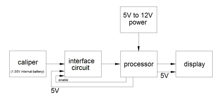
Ground, inverted clock, and inverted data then feed from the interface circuit to the processor.
