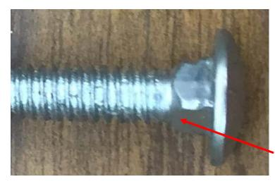
I chose to use a carriage bolt as my re-forming tool. First I put it on the lathe and used a cut off tool to square up the bottom of the head.
