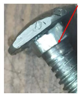
Squaring the bottom of the head with a parting tool gave me a flat surface that would contact the face of the hole.
