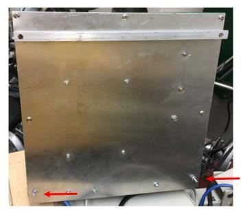
The box just hangs on the wall by a channel bolted to the back of the box. Long screws (red arrows) at the bottom keep the box parallel to the wall.
