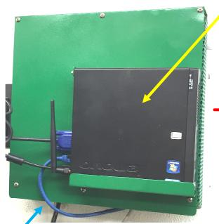
The blue Ethernet cable attached to the left side of the PC runs inside the green box to the Acorn board. My PC is a Lenovo ThinkCentre M92p Tiny preloaded with Windows 10. It has a solid state drive, 4 GB of RAM, and WiFi. Since I cannot have real time hogs like virus scan on this PC, WiFi is normally turned off.
