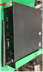
The PC sits on a custom fit shelf and is locked in place with a single screw (red arrow).
