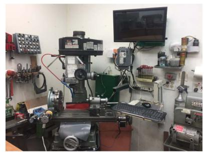
I was excited to hear that Centroid was about to come out with the Acorn<sup>4</sup>. The software that runs on a PC with Windows 10 provides the human/machine interface while a custom board called Acorn drives steppers.
