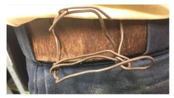
The design works well but I didn't know that initially. In the spirit of "fail fast", I bent up a model using thin bailing wire.
