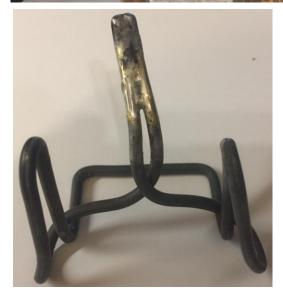
The final bends were done free form with Channel Lock pliers. Then I brazed the ends together. Going to my belt sander and 3M wheel, I rounded and smoothed the end.
