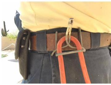
Then I got thinking about the cable relief on my edger. It forced too tight a bend in the cable but the idea was good. I have taken that basic idea, increased the loop radius, and now have a useful, if not geeky, solution.
