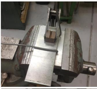
To finish the bends, I clamped down a 3/16 inch by 2 inch bar. Then I used my hammer to flatten it down. After bending one wire, I moved the clamp and bent the other wire.
