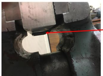
Next, I took a 1 inch by 2 inch bar of aluminum and clamped the wire in the vise.
