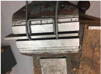
Changing to a 3/16 inch by 1 inch steel bar, I could hammer over the wires to close the belt loop.
