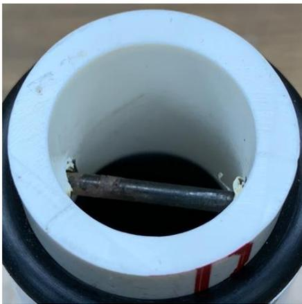
Using the outside diameter of the pipe as your gage, cut a piece of the coat hanger. Use a file to make the ends square. The goal is to push the coat hanger through the holes just formed and have the wire not stick out either side. If too short, it will fall out.
