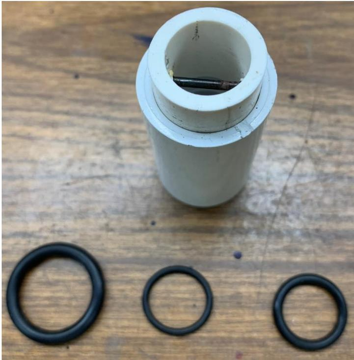
Here are the three O-rings ready for the final assembly. On the left is a number 211. In the center is a 012, and on the right is a 113. I'm no expert on O-rings, but I think these are the right numbers. I suggest you bring the adapter plus the Boston filler nozzle to the hardware store and trial fit the O-rings.
