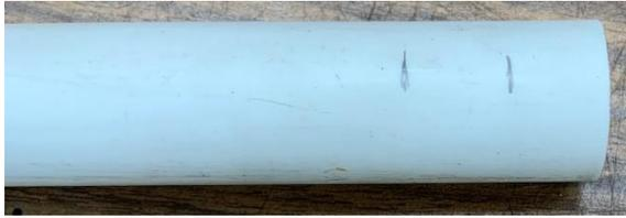
Start by marking off ½ inch from the end and 1 inch from the end with a pencil.
