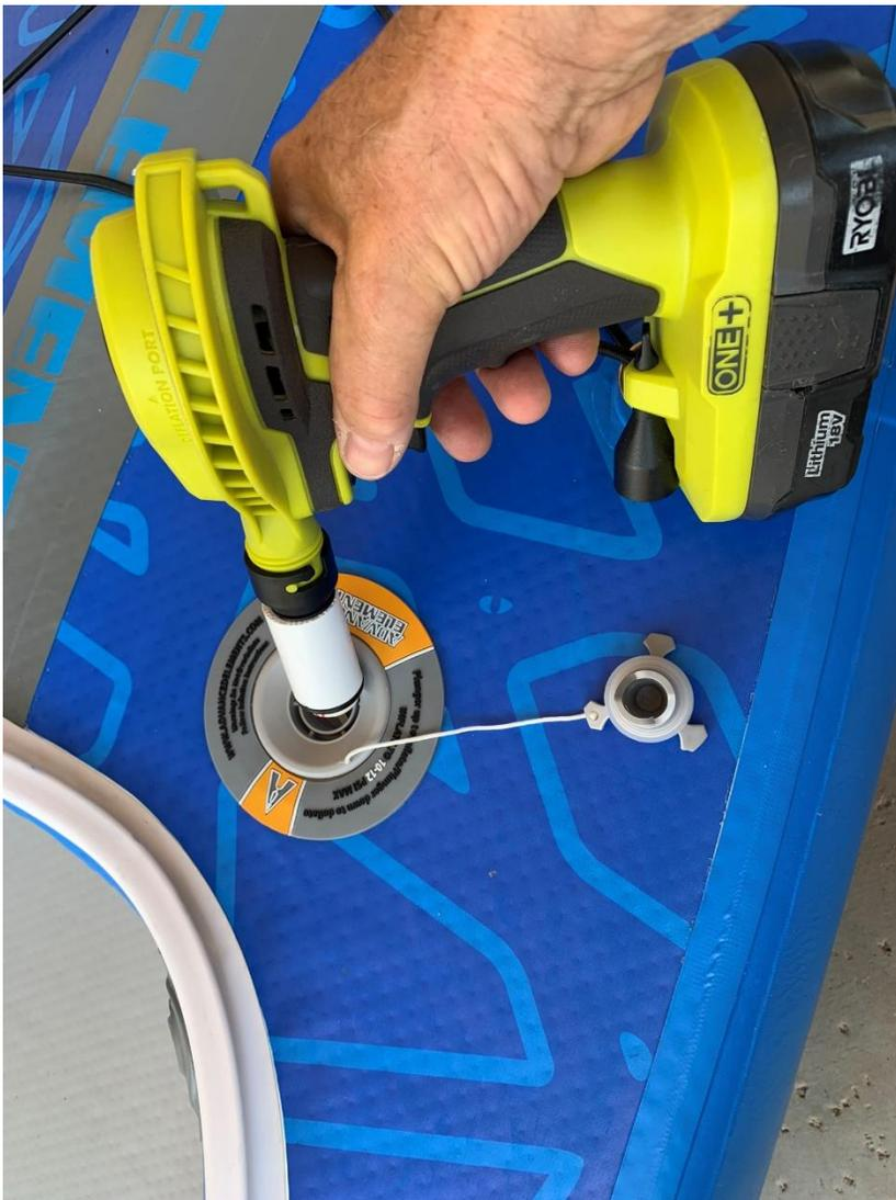
To use the adapter, take off the Military valve's cap and be sure the push button found inside is up. In this position, air can flow in but will not come out.
