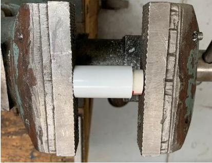
The piece of pipe is pressed into the coupler until the ends of the wire are hidden. I'm using a vise to do this task, but it can be done by pushing the assemble down on a table. Check often to be sure you don't push it in too far. Getting it back out is not easy.
