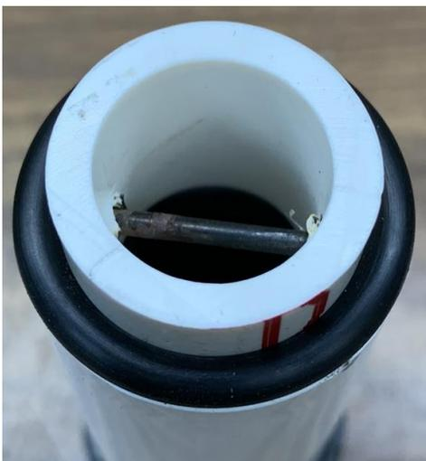
The 211 fits around the pipe. Given the low pressure, pushing this down on the Military valve provides a good seal.
