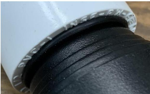
The 012 O-ring helps to center the nozzle in the bore but is not a pressure seal.
