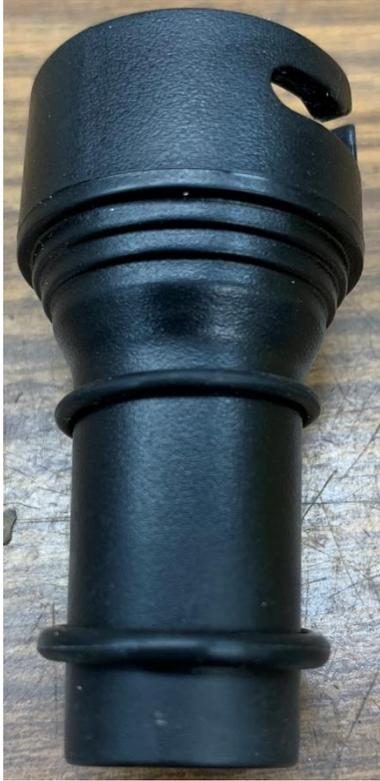
The 012 O-ring slides onto the Boston nozzle first. Then put on the 113.
