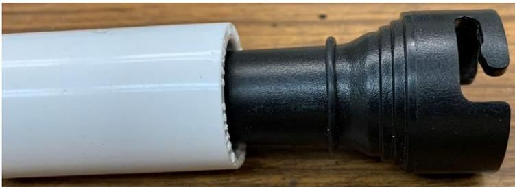
Using a twisting and pushing motion, work the end of the nozzle into the coupler. When the O-ring is all inside, straighten the nozzle and push it in.
