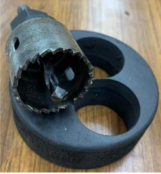
Both rubber plugs were dried out and cracked. Not to worry, I cut new ones with my hole saw and my ready supply of hockey pucks. I misjudged the height of one of the pucks so I had to make up for it on the other puck. This should not affect the operation of the bolt cutter.
