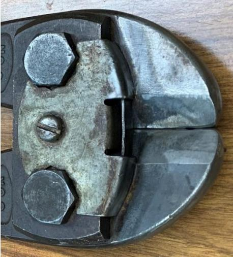
I first backed the large screws all the way out and then tightened the small screws until the jaws met when the handles were pushed almost all the way together. It was then possible to see what metal had to be filed away to return the jaws to parallel. I filed away around 0.05 inches of metal from the damaged area. A few cycles of filing, checking, and filing some more and this is the result. The jaws have about a 0.01-inch uniform gap.
