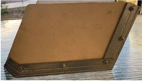
The scoop has a backbone made from a piece of galvanized steel track<sup>2</sup> used to build walls.
