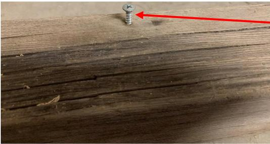
On the other side of the wood, I installed a wood screw. It is about ½-inch from the edge and is centered along the block's length.
