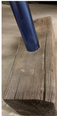
I lift up the tube, hold the bike straight up, and slide the block over with my foot. The tube drops into the hole.
