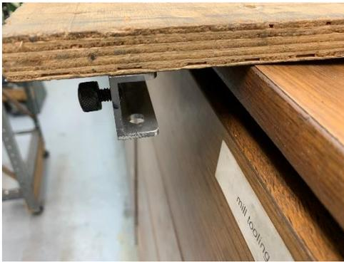
I install the shoe by sliding the channel under the front lip of the dresser. When it makes contact, the angle drops over the far edge.
