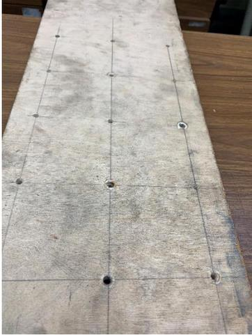
The board was first drilled 3-inches on center using a #4 drill. Then I chucked up a length of 1/4-20 threaded rod and tapped all of the holes.
