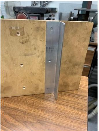
At the other end of the board is a piece of architectural extruded aluminum angle. It is secured the same way, with 3 countersunk screws.
