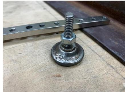
Each hold-down clamp is secured with a chair leg adjustable foot<sup>3</sup> and a Socket Head Cap Screw. To prevent screws from pulling out of the wooden threads, I screw in the chair leg bolt in about 1/2-inch.
