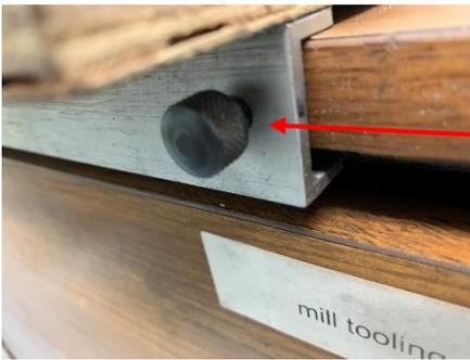
If I want to prevent the shoe from sliding sideways, I tighten this thumbscrew. I can tighten the vertical setscrew to stop the shoe from lifting.
