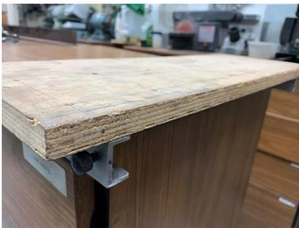
I can also slide the shoe sideways to get a clamping lip on the flank of the dresser.
