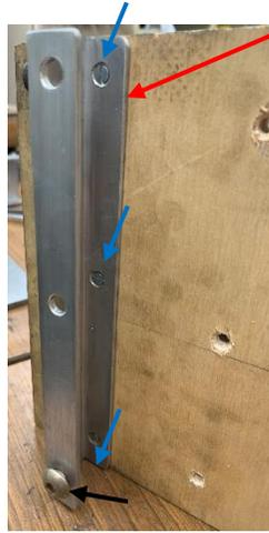
My “hook” consists of a length of architectural<sup>2</sup> extruded aluminum. It is secured with countersunk screws (blue arrows). The holes above these screws provide access for my screwdriver. The bottom access hole was tapped 3/8-16 for a vertical setscrew (black arrow). At the top, I tapped 1/4-20 for a horizontal setscrew (green arrow).
