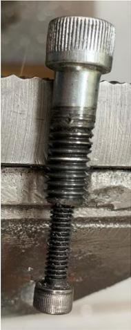
I removed the SHCS and put it on my lathe where I could drill and tap the end 8-32 to a depth of about ½ inch. There was already a through-hole in the movable jaw support which gave me access to the end of the screw.
