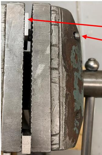
I lightly clamped the stock at one end of my vise jaws, placed the undersized packing on the other end, and finger tightened the small SHCS with a hex wrench. I then fully tightened the vise and jaw tilt was minimized.
