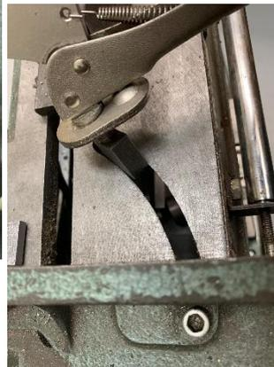
The stud's nut has been replaced with a block. I drop the block down into the table's curved slot and rotate the clamp a few degrees to lock it in place. Easy install and easy removal.
