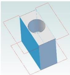
Next, I sawed the cube to the needed thickness. Since the hole was drilled and tapped first, it was easy to center it by eye between saw cuts.
