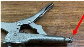
Next, I removed the metric adjustment screw from the end of the clamp and ran a 5/16-18 tap<sup>5</sup>. This permitted me to use a length of threaded rod I had in my junk drawer.
