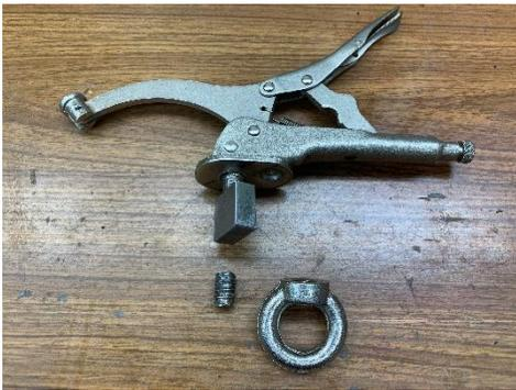
I first fabricated the stud block. My junk drawer yielded a 1-inch cube of CRS. I drilled and tapped  $\frac{1}{2}$  - 13 to a depth of about  $\frac{1}{2}$  inch. First used a tapered tap and then a plug tap.
