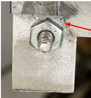
To avoid this bit of drama, I notched out a little of the large strap, so the drill is only going into the small strap. This notch was wide enough to clear the locking nut.
