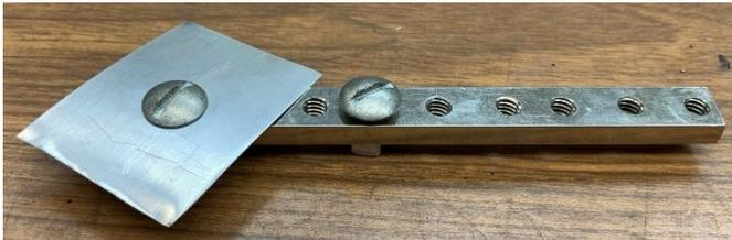
I started by playing with the idea using my prototype bars<sup>2</sup>. I quickly *re*-learned that I must support the stock at the point of cutting. Duh.
