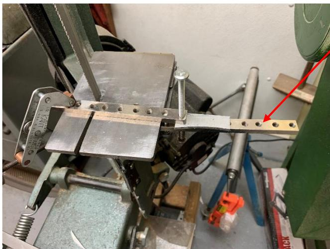
Using a second prototype bar to form a clamp on the right side of the table, I attached my proof-of-concept to my fold-down table<sup>3</sup>. A Kant Twist clamp secured the left side. As bad as it looks, the arrangement taught me that the center of my pivot point must be aligned with the teeth of the saw. Otherwise, the blade can bind, and the resulting arc will not be centered on the pivot point.
