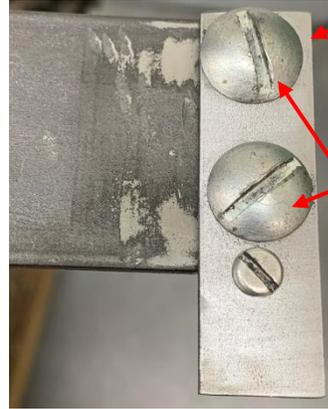
I attached a piece of ½ inch wide by 1/8th inch thick strap using two ¼-20 bolts on the right end of the tool. The wide strap was drilled and tapped while the small strap
