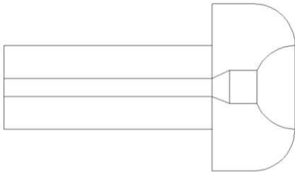
Chuckling the part by the smaller diameter end, I drilled through with my 3/16 inch drill. Then I used my 1/2 inch ball end mill to drill down about 1/8 inch. This was followed by my “F” drill (0.257 inch) down about 1/8 inch in the bottom. Nothing precise here.
