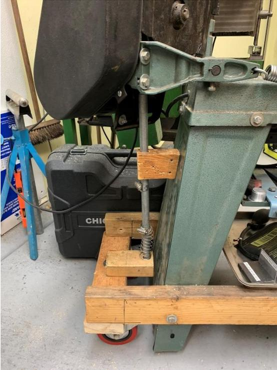
My proof of concept, and possibly my final embodiment, is shown here. When the saw's arm is raised to the vertical position, it pushes down on a length of electrical conduit.
