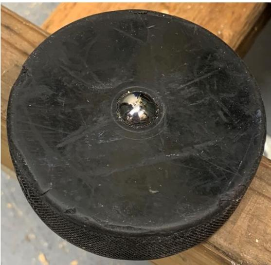
My first step was to chuck up a scrap hockey puck in my lathe. I first drilled it through with a 3/16 inch drill. Then I used a 1/2 inch ball end mill to drill in about 5/16 of an inch. Then I pressed in a 1/2 inch diameter ball bearing. It snapped tightly in place. If I had to remove it, I can drive it out through that 3/16 hole.
