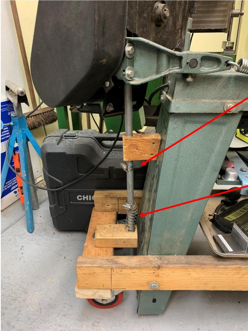
The ball joint permits the bottom face of the puck to be flat on the floor even if the conduit is not perfectly vertical. This let me slap together guides for the conduit from two wood blocks.
