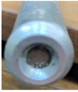
The other part of the ball joint was also turned on my lathe. Using a piece of 5/8 inch diameter scrap aluminum, I first turned the OD for a length of about 1/2 inch to be a snug fit to the inside of the conduit. Then I sawed off the part leaving about 1/8 inch beyond the reduced diameter.
