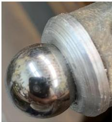
Final alignment of the magnet was performed by dropping a 1/2 inch diameter ball bearing into the socket. Then I heated up the part with a hot air gun until the glue started to flow. Next, I pushed the socket down on my bench with the ball bearing on the bottom. This set the magnet in contact with the ball and ball in contact with the socket.
