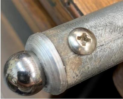
I thought heat glue would hold the socket into the conduit but it did not distribute very well so I drilled and tapped for a 6-32 screw.
