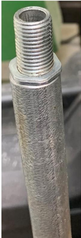
The top of the conduit was intentionally cut about 1 inch short. This let me drop a length of threaded lamp rod with a nut into the top.
