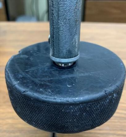
With the conduit roughly vertical, the hockey puck is free to adjust a few degrees and come into full contact with the floor. The magnet is strong enough to hold the hockey puck yet it easily releases if I want to inspect the bottom face. I suspect that swarf will embed itself into the puck and will have to be periodically cleaned.
