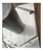
Here you see that the 0.750" diameter drill rod does fit into the milled hole. It is not possible to see even in this magnified view, but there are two crescent shaped slivers
