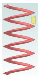
Look what happens when we change the direction of rotation of the lead screw. The threads move away from the nut and they are no longer in contact. As you turn the lead screw crank, there is almost no resistance. The table stops moving. Keep turning and eventually the thread will again contact the nut. Over some number of degrees of rotation, nothing happened.
