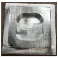
Due to various false starts, I ended up making this test coupon a half at a time. One coupon has the perimeter of a  $1-1/2 \ge 1-1/2$ " square milled correctly. The other had the hole.
