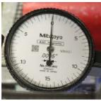
At this point, I zeroed the X axis Digital Read Out (DRO) in Mach3 plus zeroed the DTI.
