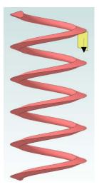
When this helix is turned counterclockwise as viewed from the top, the yellow nut is pushed down. As long as there is contact between thread and nut, the nut will move down at a rate entirely determined by the rotation of the helix.
