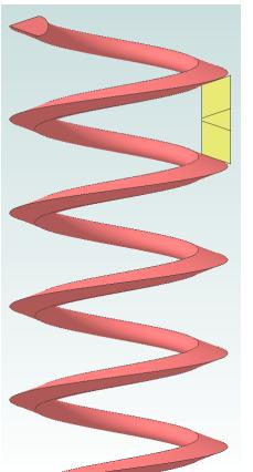
The orange helix is the thread of the lead screw. The yellow block is part of a nut. In this case, the nut is a snug fit to the thread. Assuming both thread and nut are perfect, there is constant contact between them as the thread is turned in either direction.
