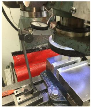
I set up my finger Dial Test Indicator (DTI) so the base was supported by the mill's table. The finger rested on the lower spindle bearing housing.
