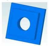
So far we have been addressing just the first "layer of the onion". The second layer includes actual cutting forces. An elegant test was suggested by Steve "pilotltd". A square perimeter is side milled followed by a hole in the center. By comparing the lengths of the sides of the square, we can see how well cutting along the X axis compares to cutting along the Y axis.
