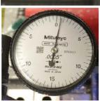
I next jogged one *negative* step at a time while monitoring the DTI. As soon as the DTI dial moved, I stop pressing the step button. In my case, the dial moved about +0.0005". That is enough to tell me I am through the backlash zone plus went 0.0005" over.
