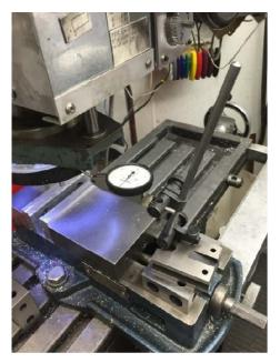
The Z axis is different from X and Y axes because there is a spring that lifts the quill. This ideally eliminates backlash. But there is still backlash in the drive mechanism. Using the procedure, I found a backlash value of 0.0014" worked.
