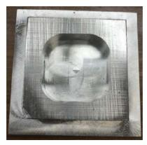
In the first test coupon, I milled a pocket 0.300" deep. Using my best mic, I zeroed it on the face of the square. Then I moved the mic into the pocket and read -0.30775". This is an error of 8 thou! Clearly there is more work needed on the Z axis.
