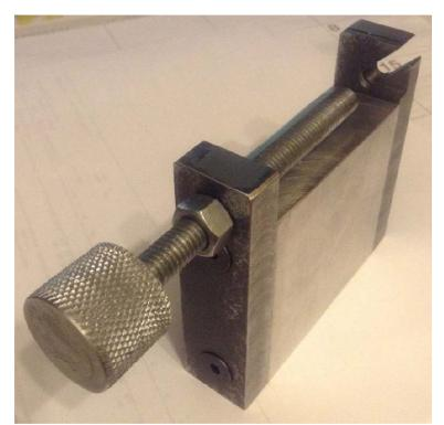
This fixture lets me cut ½-20 bolts on my horizontal bandsaw quickly and safely.
