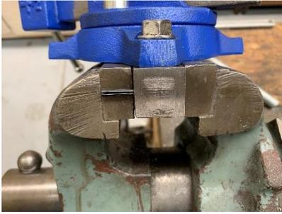
These roll pins eliminate an annoying problem. I can only rotate the jaws of the large vise when they are not clamped down. So when I am rotating the main vise jaws with the auxiliary vise on top, the auxiliary vise will tend to slide.
