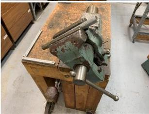
Once in a while, I need to work at other than horizontal. My vise pivots all the way to the jaws being vertical.
