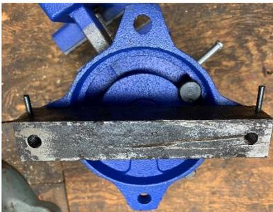
The final step was to drill 1/8 inch holes 0.15 inches from each end. I drilled in about 1/2 inch. Roll pins were then pressed in place.
