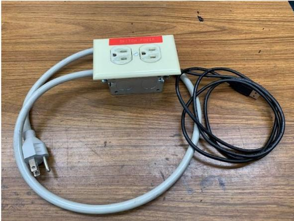
With the sides reattached to the box and the cover installed, I added the label “SWITCHED POWER”.
