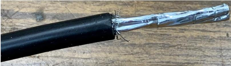
Trim off all of those fine wires and carefully inspect the cable to be sure they are all removed. Even one of these wires would cause far too much excitement if it happened to touch the 120 VAC wires.
