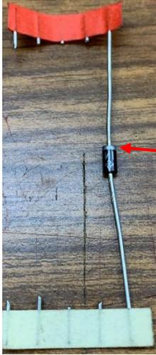
Any small diode will work in this circuit. The only requirements are that you can see the band painted on its body and that it fits across the relay.
