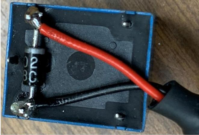
Solder the diode and wires to the relay pins.
