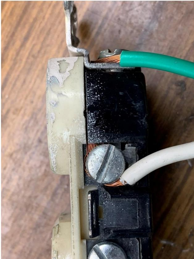
The green wire from the power cable has about ½ inch of insulation removed. Twist the strands tightly together and clamp them under the ground screw of the outlet.
