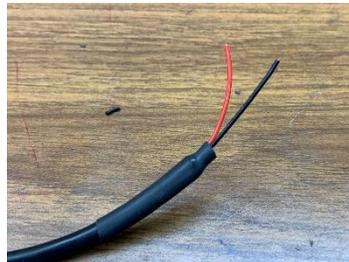
A few seconds with a heat gun and the end of the USB cable is nicely insulated.
