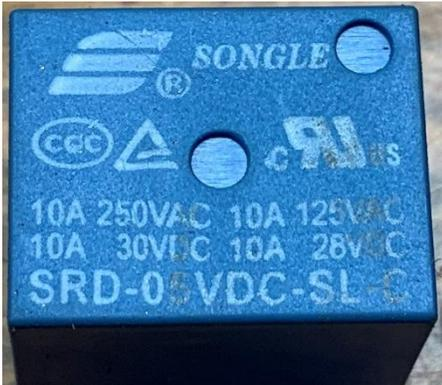
It came as a nice surprise to learn that many modern appliances use a **relay** that can switch up to 10 amps at 120VAC with a coil that only needs 5VDC. This means low cost. I bought 10 of these beauties on Amazon for \$7.86 with Prime<sup>3</sup>.
