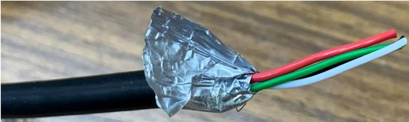
Unwrap the foil to expose the 4 wires.
