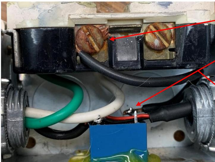
A short length of black wire is secured under a screw that is adjacent to the shorter slot of the outlet and connects to a pin on the same side as the red wire from the USB cable.
