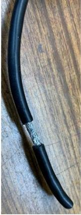
I need to expose two wires from within the USB cable. Step 1 is to carefully cut off about 1 inch of the outer insulation. You will see a braid of very fine wires under it.
