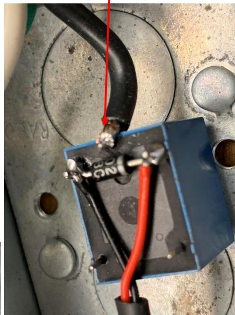
Now would be a good time to glue the relay to the bottom of the outlet box.
