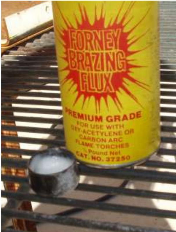
I used Brazing Flux because it was at hand. Note the mixture of flux and water in the little black cap. Water was added until I had a paste. The water will boil off early in the splicing process so it only used to hold the flux in place until heat can start to melt the flux.
