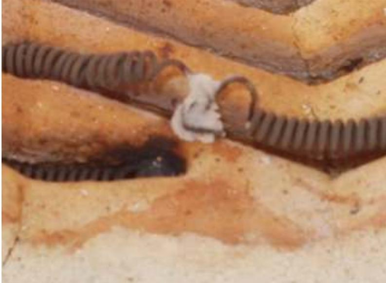
I've just slathered some of the paste onto the hooked ends. Some attempt was made to align the ends so if this worked, I would be able to stuff the element back into its slot.
