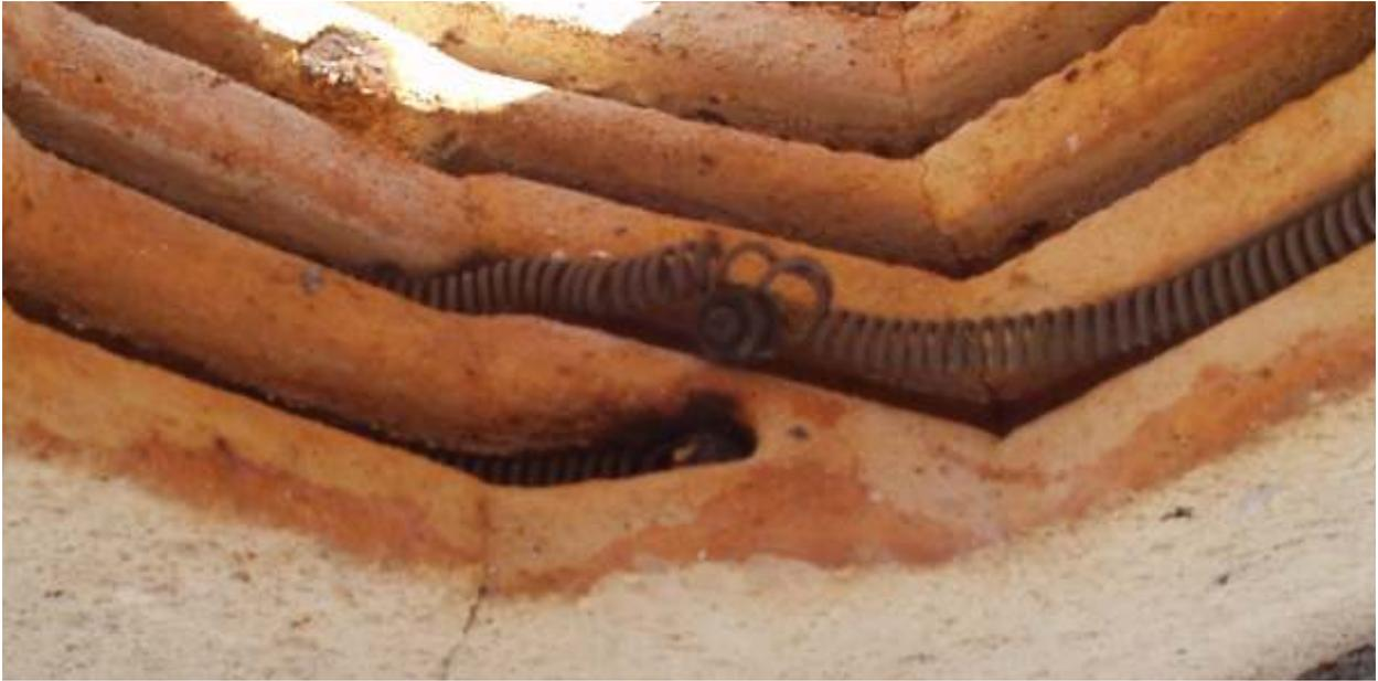
Here you see the ends of my heating element lifted out of their slot. Hooks have been formed in the end.
