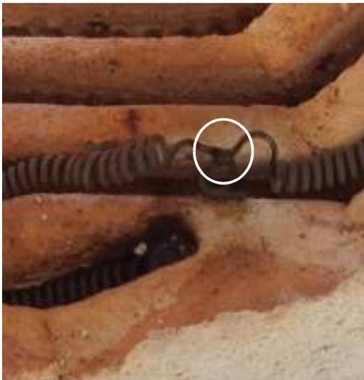
This is not the best picture but hopefully you can see the thickened area where the two ends were hooked inside the white circle. The splice was strong enough to push down into the element's slot.
