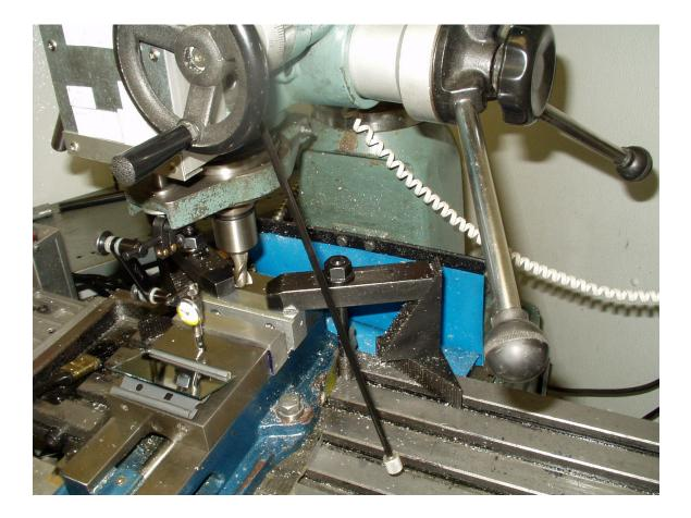
I have removed the set screw from the graduated collar and screwed in a rod. At the end of the rod is a scrap knob which makes it easier to lock the graduated collar to the downfeed shaft. The bottom of the rod just clears the lip of my vise base. By far, the hardest apart of this construction was putting a coat of black paint on the rod to make it look nice. When not in use, I unscrew the rod and put it aside.
