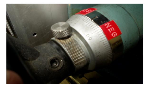
My downfeed handwheel has a graduated dial on the same shaft which can be locked in place as needed via a set screw. One full rotation causes the quill to move almost exactly 0.100". How accurately I can set a given position really depends on how well I can creep my fingers along the circumference of the handwheel.
