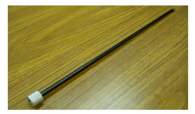
Find a length of scrap 1/4" rod, hopefully with one end already threaded to match the set screw. Mine is 1/4-20. If necessary, cut the rod so the bottom clears at least the mill table. Then find a knob for the other end. If you really want to go crazy, paint the rod. That's about it.
