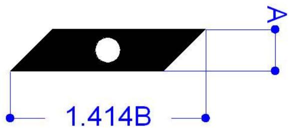
The PTN has a width of "A" although making it 0.02" thinner will make it easier to drop down the T slot. The length should be 1.414 times the width "B". In this way the angle is a simple 45 degrees. The hole is tapped  $\frac{1}{4}$ -20. The thickness of the PTN is limited by the T slot but I happened to have  $\frac{1}{4}$ " plate. This seemed reasonable given I am using a  $\frac{1}{4}$ " diameter bolt.
