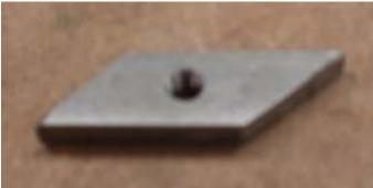
I made just one PTN to test out the design. To make a bunch of them, I would start by cutting the bar's width to A-.02". Layout the 45 degree lines every 1.414 times B inches with a little extra for the saw's kerf.
