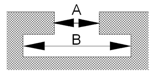
A regular T nut may have a  $\frac{1}{2}$ -13 thread which engages metal almost "B" wide. The PTN is limited on its width because it must fit through "A" so can't handle more than about  $\frac{1}{4}$ -20. Going larger would mean little metal flanking the hole.
