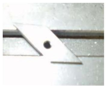
Here is a prototype of the T nut invented by Nanda. I placed it over the T slot so you can see how it works. The width of the Parallelogram T Nut (PTN) is slightly less than the width of the T slot.
