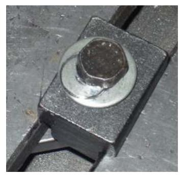
I used a standard T-nut as my top support, put a washer on top, and dropped a 1/4-20 screw down the hole. You can see the PTN in the slot.
