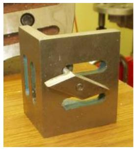
The PTN is ready to clamp down a small angle plate. There is room to add a second PTN if necessary.
