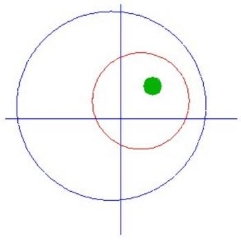
We then end up with a situation like this one. The blue circle is the spindle and its center is not on the center of rotation. The red circle is the body of the EEF. The green dot is the end of the EEF's pin. Nothing is lined up with the center of rotation. This case is not all bad because it enables us to reduce the total TIR.
