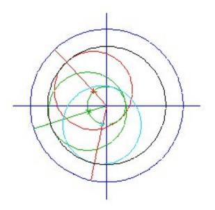
Time for a diversion to the practical. Say the blue line represents the spindle of a vertical mill as viewed by looking up. The red circle represents and end mill. A *really* bad collet holds the end mill so it turns way off center.
