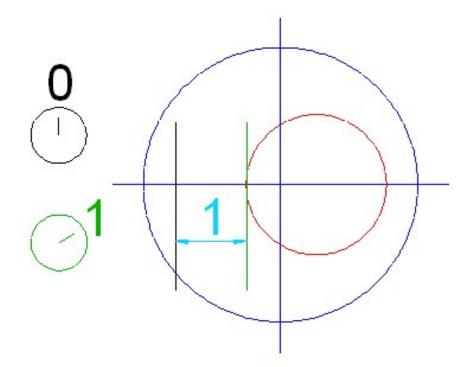
Now rotate the blue circle 180 degrees. The red circle will again have its center on the same line as the blue circle's center and the DTI's spot. The DTI will now read a minimum.
