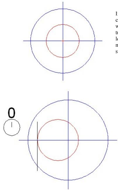
If you placed a DTI on the red circle in the ideal case, the reading would be constant as the circle turned. When I get this result in my less than ideal world, it usually means the DTI is broken, hitting a stop, or not touching the circle.
