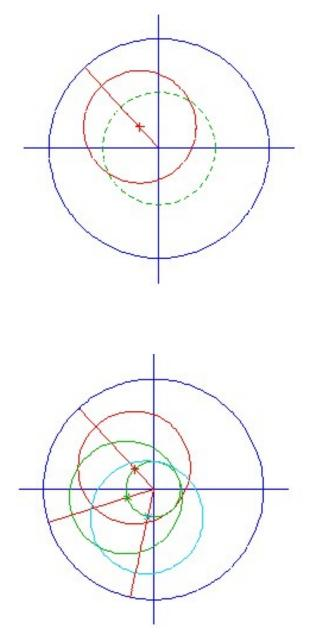
Look what happens if the red circle's center is not aligned with the center of the blue circle. The dashed green circle is its previous, ideal location and the red circle is the new location. The center of the red circle is marked with a red X. I can always draw a line from the center of the blue circle, through the center of the red circle, and out to the blue circle. This line will always be a radius.
