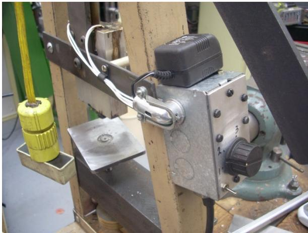
The wall wart is plugged in on top of a standard duplex AC box. Power comes in from the black cord at the bottom. The lower left corner of the front plate is my on/off switch. The fuse is inside. Not visible on the lower right corner of the front plate is the LED. The dial has 1, 2, and 3 marked on it. “1” is about 175°C, “2” is about 208°C or 33°C more than “1”. “3” is about 241°C.
