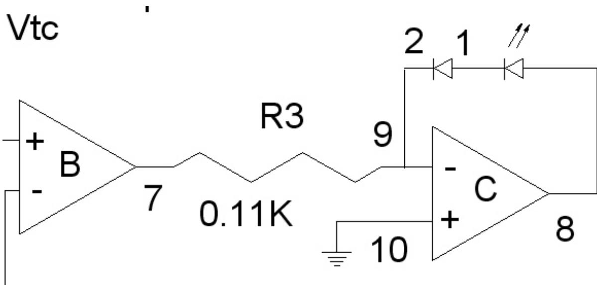
The comparator (B7) feeds the voltage to current converter made up of R3 and op-amp C. The current converter's output is between pins C8 and C9. When the comparator's output (B7) is at -4V, op-amp C is able to hold pin C9 very close in voltage to what it has on pin C10. This puts 4V across R3 so the current through R3 is  $4V/0.11K = 36 \text{ mA}$ . This current flows through the LED (marked with the double arrows) and the input of the opto-TRIAC (marked with pins 1 and 2).
