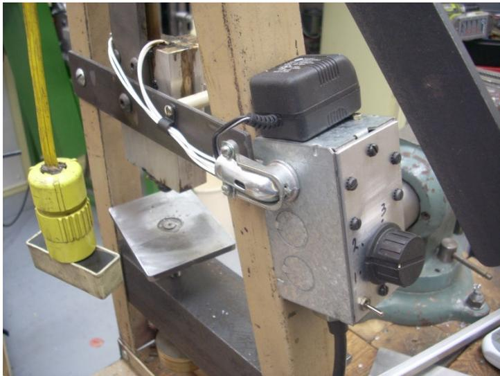
This article describes the temperature controller that I use on my modified Gingery Injection molding machine. The original design used a thermal/mechanical temperature controller which sensed the surface of the heater block. My controller monitors the temperature closer to the melting chamber. If you were to
