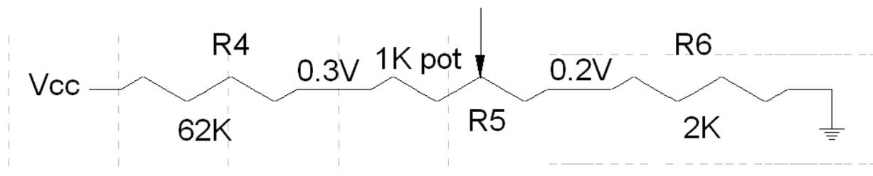
Below the comparator (B) is a voltage divider formed by  $R4$ ,  $R5$ , and  $R6$ . One end is connected to  $V_{cc}$ , our most positive power rail. The other end is connected to circuit ground.  $R5$  is a 1K potentiometer. When turned all the way
