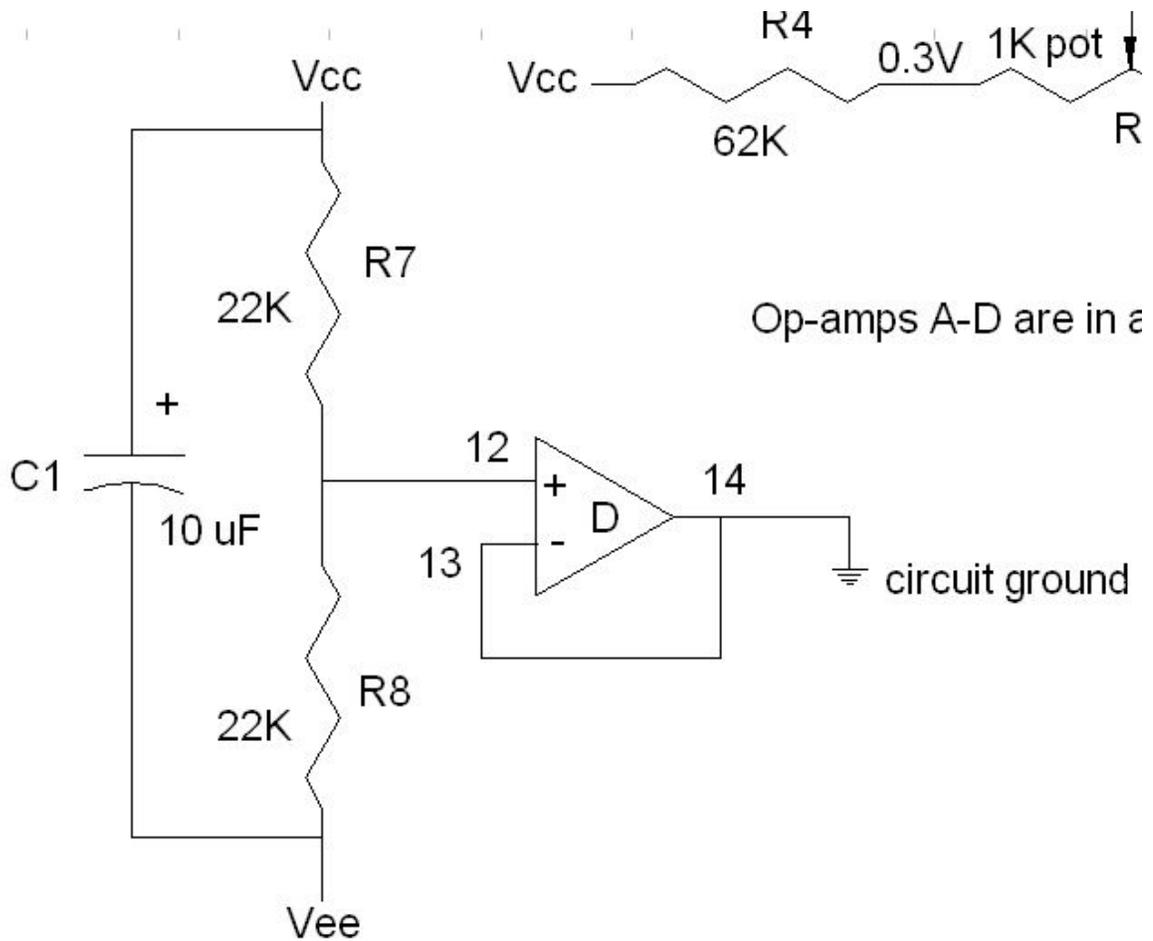
The last bit of circuit is possibly the strangest. A number of points in the temperature controller need a ground reference. In this case, "ground" simply means a voltage half way between Vcc and Vee. R7 and R8 are a voltage divider that defines this voltage. I then use op-amp D to buffer this voltage and generate
