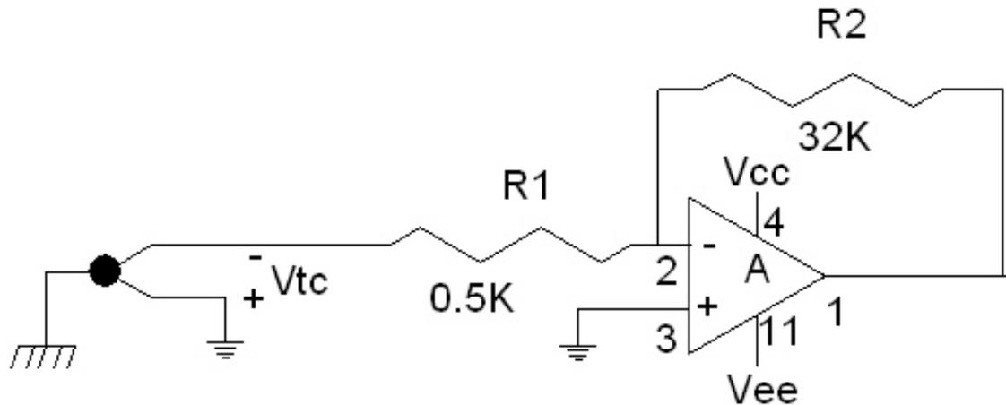
The gain of the voltage amplifier equals  $R2$  divided by  $R1$  or 64. The exact gain is not that important because of the external calibration. There is also a voltage inversion but this has been taken care of by my definition of the input voltage,  $V_{tc}$ . As  $V_{tc}$  gets larger, the voltage at pin (A1) becomes become proportionally larger and of the same polarity.
