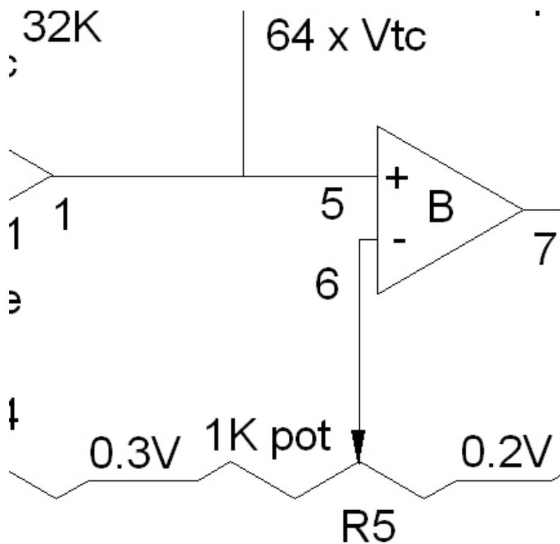
of wiper voltages. This arrangement enables me to use the entire range of the pot to set all useful temperatures. The center of this range and the limits were found empirically once I got the circuit controlling the temperature. In my particular circuit,  $V_{cc}$  is about +6.67V.
