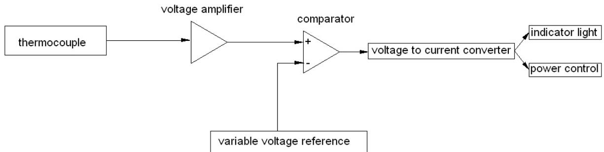
The controller is a simple “bang-bang” analog feedback system. This means that when the temperature is below a threshold, power is applied to the heaters. When above the threshold, power is removed.
