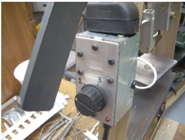
Now you can see the LED in the lower right corner of the front plate. The white wire on the right side is from the thermocouple. This wire feeds into the square tube in the background. This tube holds the splice to solid wire that connects to the thermocouple. The thermocouple is held in a spring loaded
