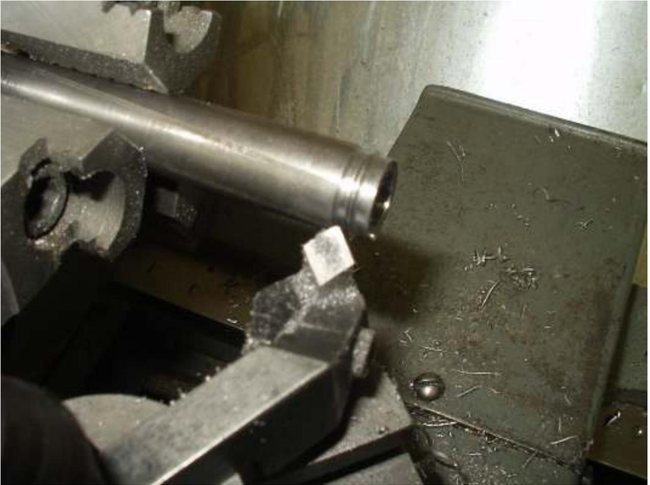
I moved the cutter so it was now 1/4" from the end. The lathe was started and I again fed in about 50 thou. This time I cut towards the tailstock until the cutting edge was fully formed. I then changed to a cut off tool and parted the washer off. As long as there was enough of the 5/16" hole down the center, I could just run in the end mill to form the cup and then use the cutter to form the ridge. Switch to the parting tool and the piece was done.
