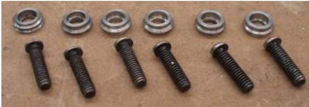
Along the top you see a set of cup like washers. They have a ridge around their perimeter that can cut into the metal being held. The screws started as button head screws but have been machined so the heads are eccentric. These screws have a hex hole in the top and are driven with an Allan key.
