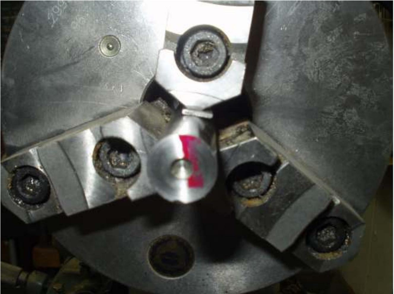
I started with a piece of 12L14 bar stock in my 3 jaw chuck. Note the 50 thou spacer between the top jaw and the bar. This provides me the 50 thou offset that will later enable me to cut the screw heads eccentric.
