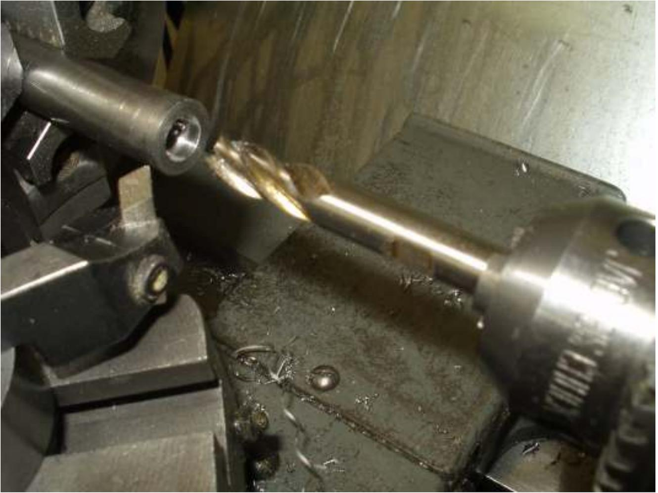
To form the cup, I put a 3/8" 4 flute end mill in the drill chuck. I went in about 1/8".
