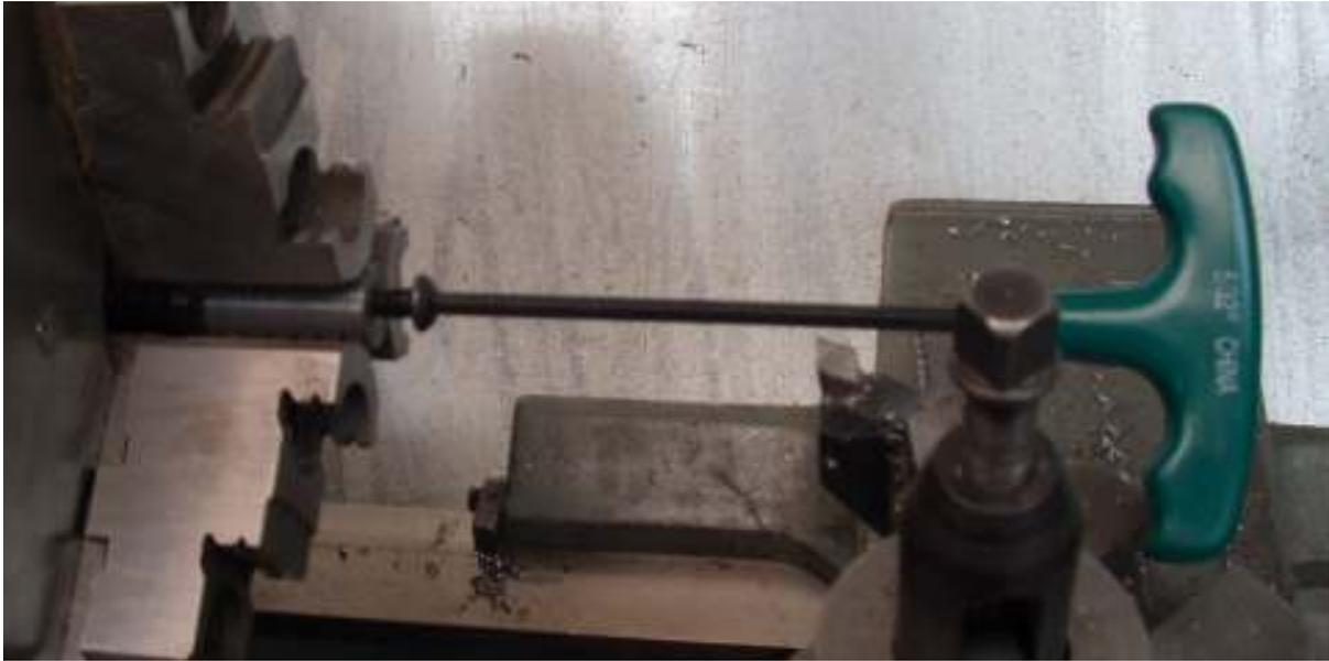
These button head screws have a hex hole in the top. I turn the screw into the fixture until it bottoms. The cutting force keeps the screw solidly against the top of the set screw.
