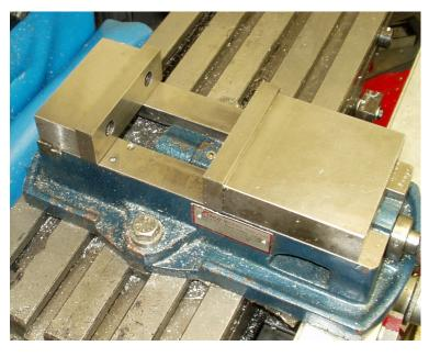
For over 15 years I have used my Enco<sup>®</sup> copy of a Kurt<sup>®</sup> vise with a good measure of success. Using my modest selection of parallels, I have been able to accommodate a variety of parts for machining.
