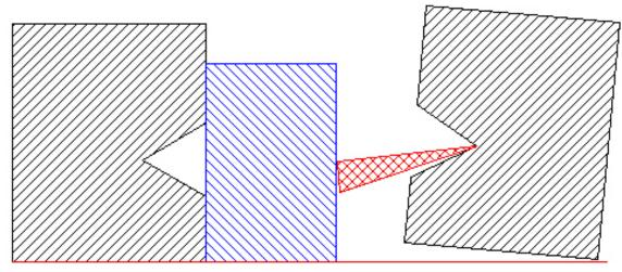
The rising of the movable jaw causes the triangle block to tilt down. This downward force combined with the closing force of the vise will tend to hold the block against both the fixed jaw and the vise's ways.
