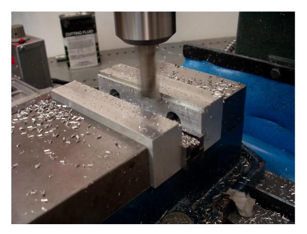
Here you see the finish cuts being made. My rough-cuts were .095" deep and .095" wide. Both jaws are cut at the same time. Then I lowered the cutter by
