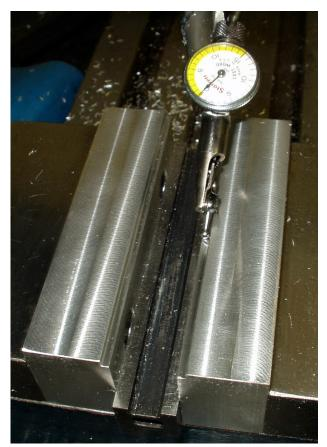
Since the step is cut in place, it must be dead true. The bottom of the step must be parallel to the table while the vertical part must be parallel to the X axis. If the mill's head is property trammed, the vertical part should also be parallel to the Z axis. Just to convince myself of this fact, I ran my Dial Test Indicator along the bottom of both steps. The needle did not budge until it fell off the far end. Both steps read the same within the accuracy of my DTI.
