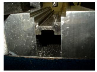
2. Ian suggested I cut the horizontal surface of the steps with a dovetail cutter. It will cut a relief in the vertical face. Then follow up with an end mill to true the vertical faces. The relief avoids the fact that a step cut with an end mill will most likely not have a perfectly square corner. Any curve at this corner will prevent
