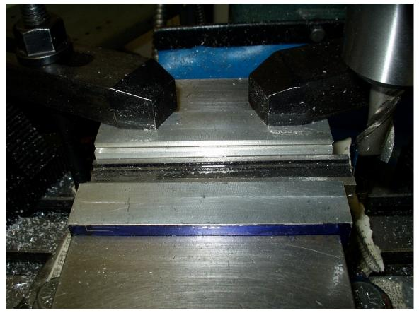
torque wrench when clamping the jack block and recorded the applied force. Then when I went to clamp the block to be cut, I used the same amount of torque. Over tightening can cause distortion and error.
