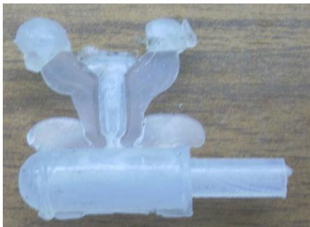
The plug is now exposed. Removing the flash takes just a few seconds with diagonal clippers.
