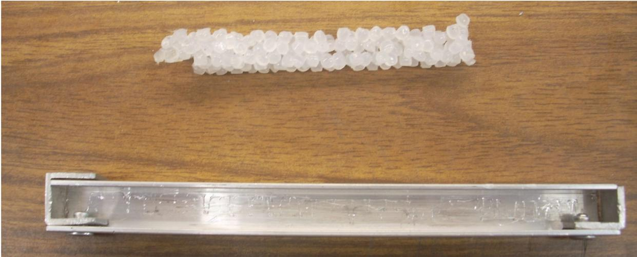
Before I can inject molten plastic, I must first load my machine with polypropylene pellets. These pellets do not pour easily into the heating chamber. They just stick to the opening. My solution is to scoop up some pellets in this rectangular box. I then heat the box to around 400° F so they partially melt and stick together. The result is an easily managed bar. I can drop sections of this bar into the chamber with little fuss.
