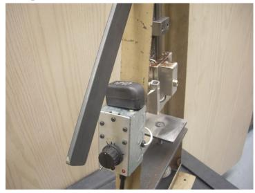
I saw nothing wrong with the temperature controller specified by Gingery but wanted to make my own. Starting at the heater block, I have a thermocouple fitted into a hole and clamped in place such that some expansion is permitted. The tip of the thermocouple is in direct contact with the heater block in a hole between the melting chamber
