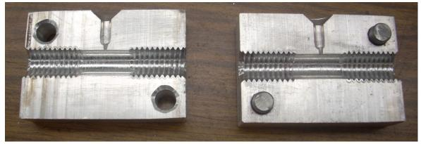
On occasion I splice a connector with associated wire to a "wall wart" that had a different connector on it. No matter how much heat shrink tubing I use, the connection is always mechanically weak. A cast cylinder of plastic around the joint would be nice.
