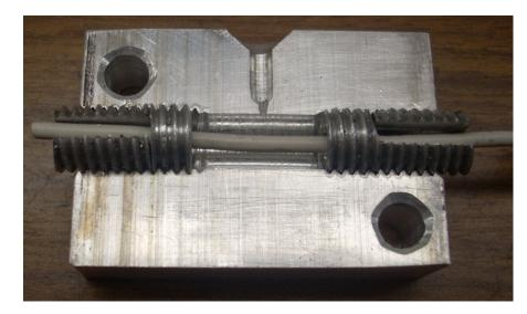
A second set of slotted slugs can be dropped into the mold in front of the first set. They help to block the molten plastic from leaking out the slot.
