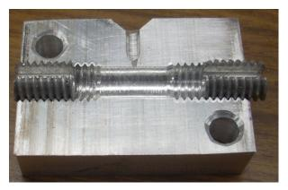
I made a pair of threaded plugs that fit the mold. Each plug was drilled out with a 1/8" diameter drill and then I milled down to the hole with a 1/8" diameter end mill. The result is a slot in each plug. The plugs can be moved within the mold to vary its volume.
