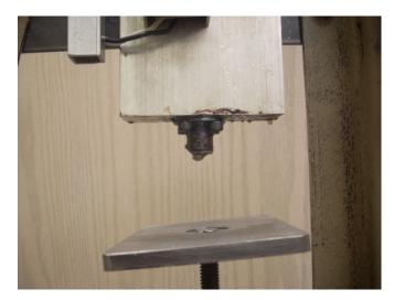
The plate below the nozzle is free to wobble. This permits the mold that is pushed up against the nozzle to align. The nozzle has a taper cut in the bottom. My mold has a countersink hole in the top. Alignment is quick and accurate.
