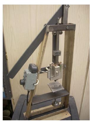
Just before shut down, I lower the plunger into the heater block. Small bits of plastic coat the guide block, plunger and heater block. Once cooled, the plunger is frozen into position.
