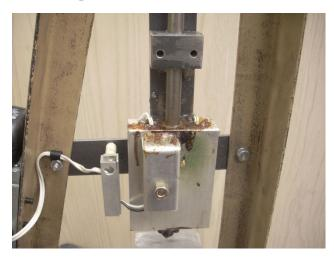
Below the ball bearing guide is my original plunger guide. It is a block of mild steel drilled and reamed for a close fit to the ½" diameter plunger. The plunger fits into a drilled and reamed ½" hole in the aluminum block. This block gets rather hot yet I don't want to also heat the frame. To minimize this heat loss, I have a piece of "FR-4" epoxy glass circuit board material between block and support frame.
