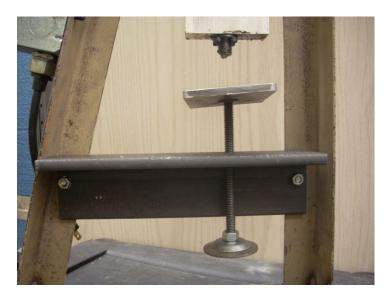
Nothing fancy here. I just took a piece of threaded rod and put two nuts and a fender washer on the lower end.
