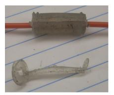
People have suggested doing one molding that will support the wire and a second molding that will encase it. Early trials show that the first molding does not fuse to the second mold. You can barely see the gap in the mold around the red wire. This gap was filled with the sliver of plastic laying in front.
