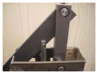
I added a pair of ball bearings to support the top of the plunger and now the machine works well. Side force on the plunger is greatly reduced but not eliminated.
