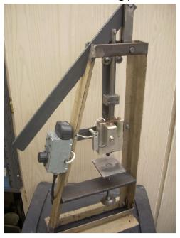
mold polypropylene around wire splices.
