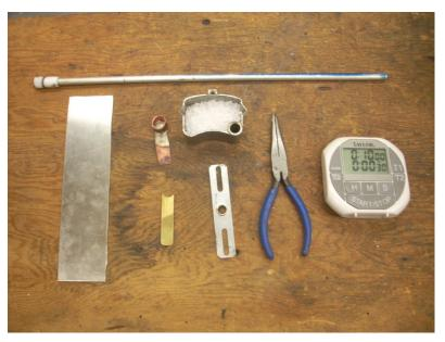
I have a few tools that help in the operation and maintenance of the machine. Starting on the far left is a plate of stainless. When I'm done using the machine, I inject the unused plastic onto this plate to create a long string of plastic. When cooled, this string is easily stored. When I wish to recharge the machine, I feed this string
