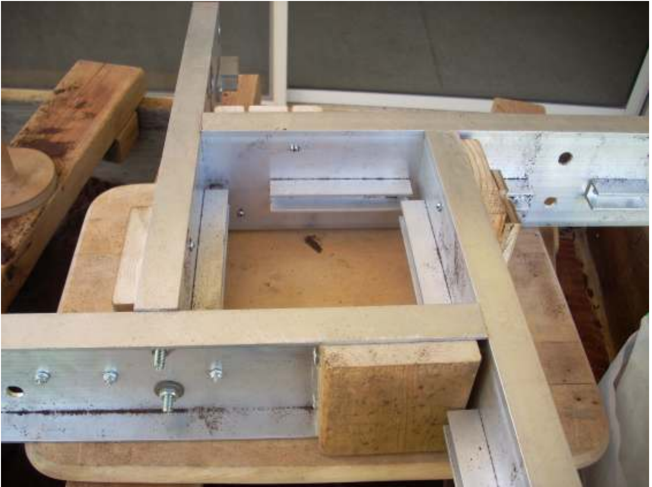
Here we have the drag on a molding board ready to be rammed up. The flask is set for minimum volume.
