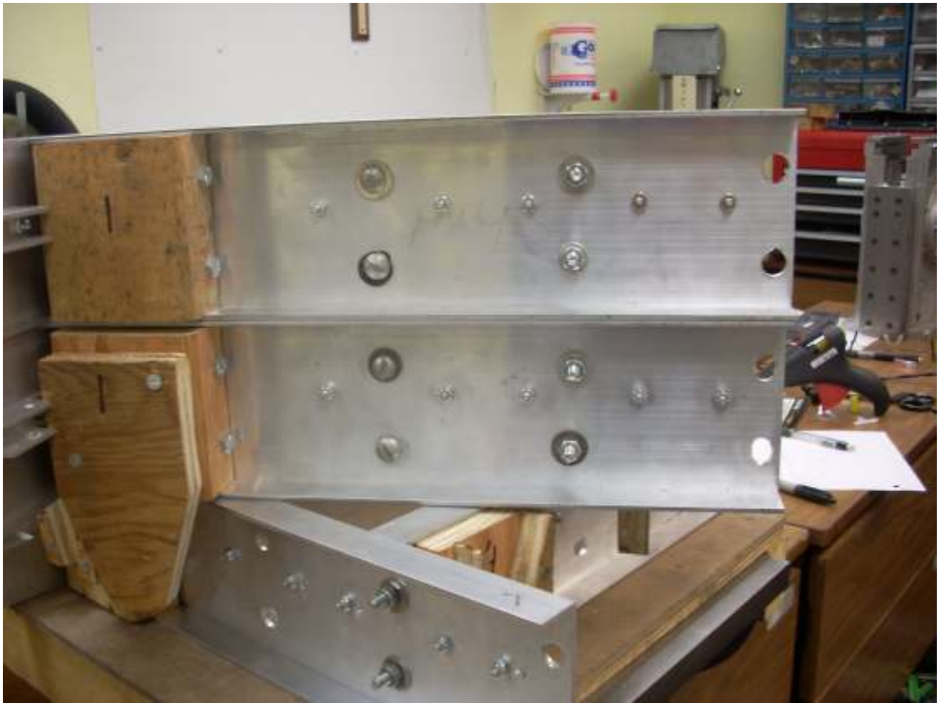
Here is the cope with my upset attached. Unused holes in the sides accept bolts that fasten bars vertically. Note the slotted head bolts above.
