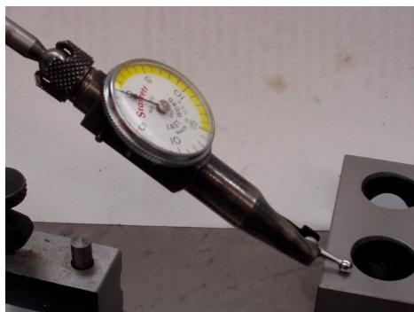
Stop for a moment and think about the repeatability and accuracy of a finger type Dial Test Indicator. Its value comes from being able to consistently tell you when the finger is in the same position relative to the indicator's body. This is an extremely useful
