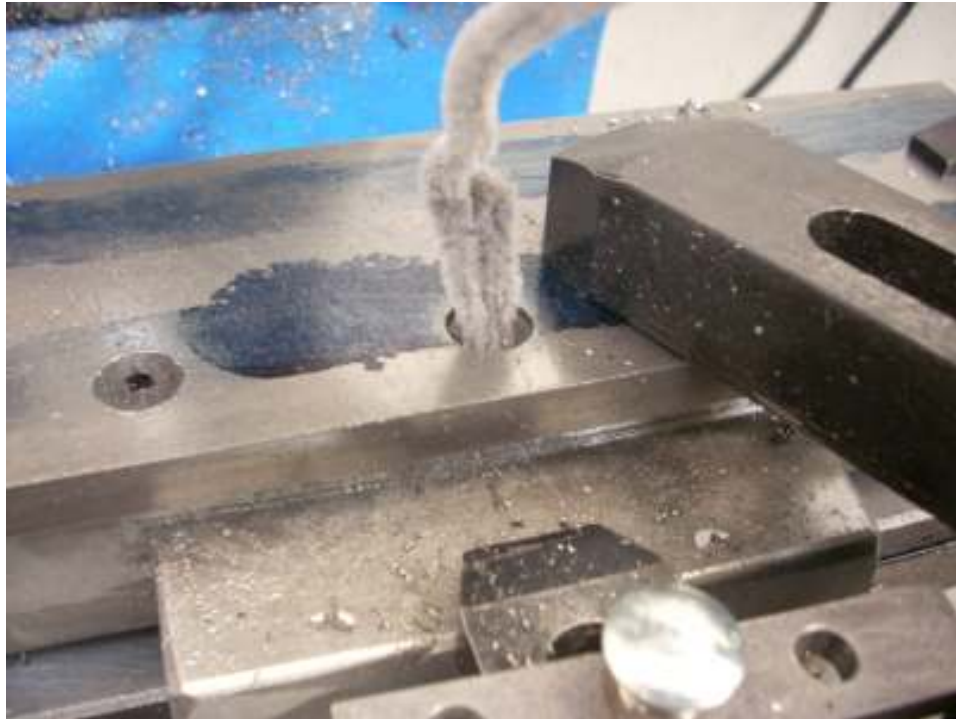
A fat pipe cleaner was used to remove swarf from the threads. Some swarf has been jammed into the bottom of the hole but it is harmless
