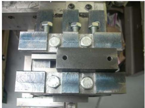
This arrangement did not work very well. The vise jaws would not grab the table. I think this is because the table was cut with the shaper and so has tiny ridges on it which greatly reduce clamping friction. Don't worry, I fixed this later.
