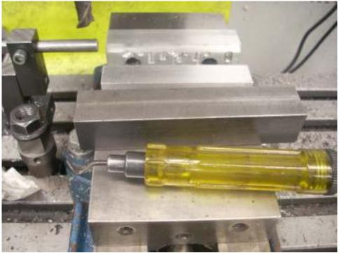
The top face is cut, deburred, and then rotated so it sits against the fixed jaw of the vise. The cycle repeats until all 4 sides are square. The exact dimensions of the block are not important but it is critical that it be square and that I take the same amount of material from each face to minimize warpage. I took 0.004" from each face.
