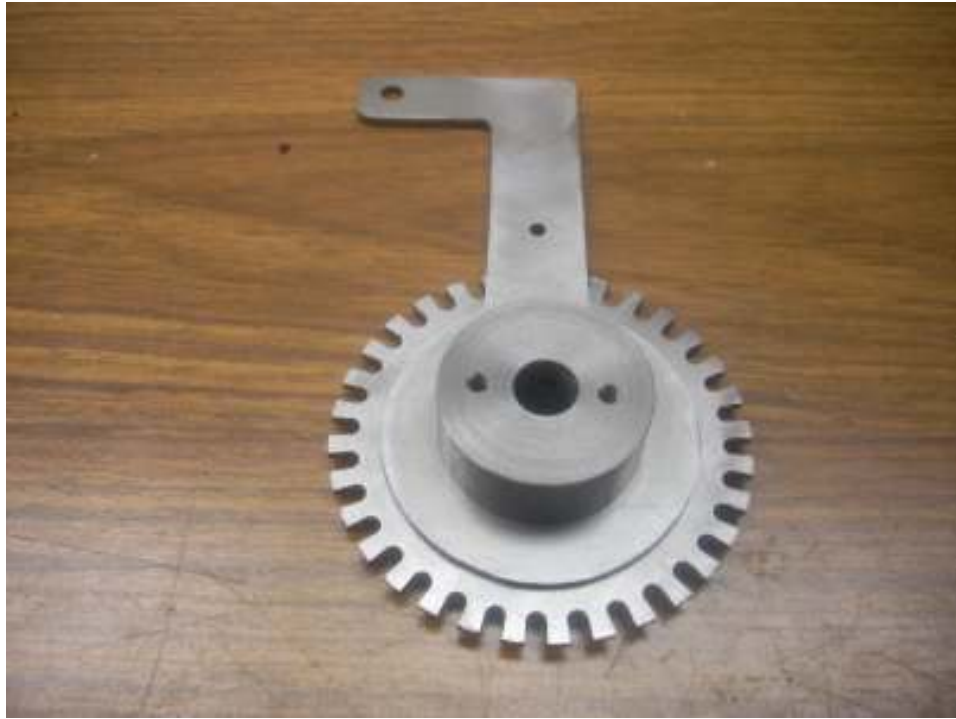
The ratchet plate is a smooth sliding fit on the hub.
