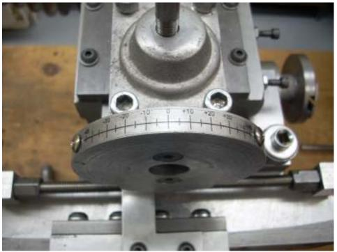
The scale was then attached to the protractor using 6-32 screws.
