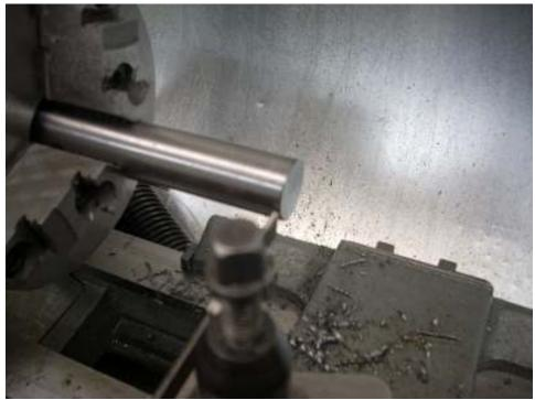
After squaring off the end, I used a parting tool to cut a groove for the D ring.
