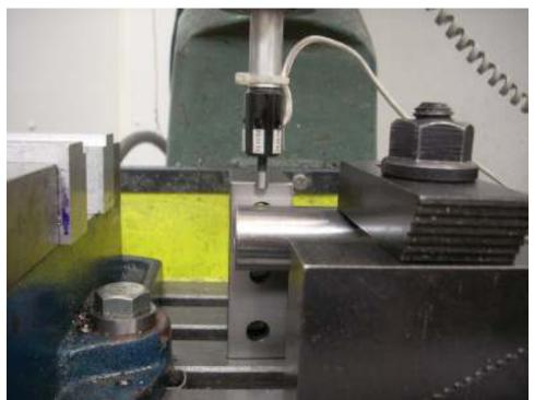
The pin was set up on V blocks on my mill. I used my edge finder with a 1-2-3 block to locate the side of the rod. Then I dialed over 0.500" to find the centerline.
